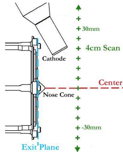
Figure 6. Test Orientation.
