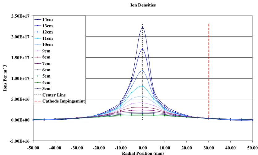
Figure 9. Faraday probe test data.
