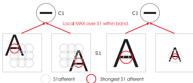
Figure 2: How scale and position tolerance is gained at the C1 level: Each C1 unit receives inputs from S1 units at the same orientation ( e.g. , 0^\circ ) arranged in bands . For each orientation, a band \Sigma contains S1 units in two different sizes and various positions (grid cell of size N^\Sigma \times N^\Sigma ). From each grid cell (see left side) we obtain one measurement by taking the maximum over all positions: this allow the C1 unit to respond to an horizontal bar anywhere within the grid, thus providing a translation-tolerant representation. Similarly, taking a max over the two sizes (see right side), enables the C1 unit to be more tolerant to changes in scale.
