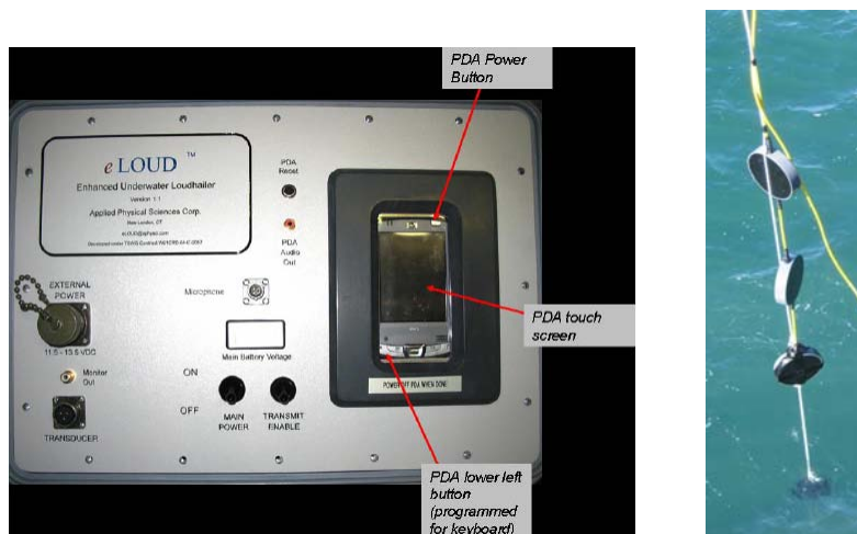
Figure D-1. The photographs show the control unit and the vertical three-transducer array just prior to deployment (photographs courtesy of Bruce Abraham, Applied Physical Sciences Corporation).
