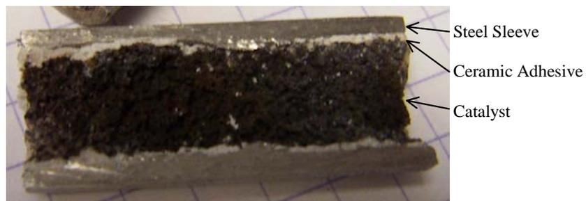
**Figure 10: Section of Catalyst Bonded into Sleeve**
