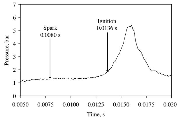
**Figure 9. Spark-ignited tube head pressure trace.**
