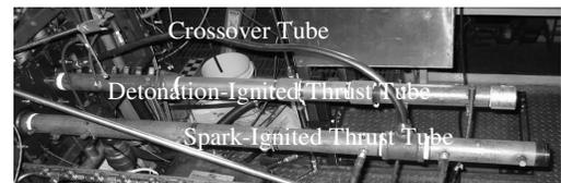
**Figure 5. Thrust tubes and crossover tube.**
