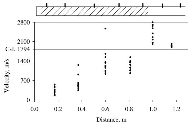
Figure 7. Spark-ignited thrust tube and corresponding wave speeds.
