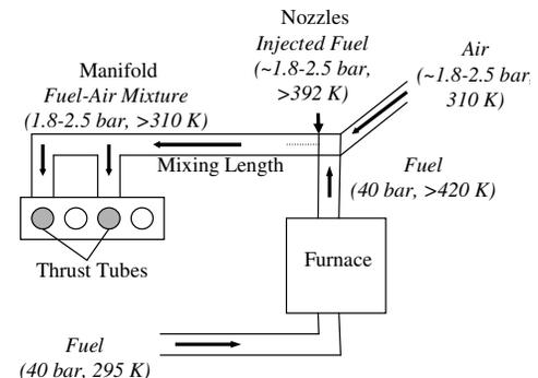
**Figure 4. Vaporization system schematic with temperatures and pressures.**
