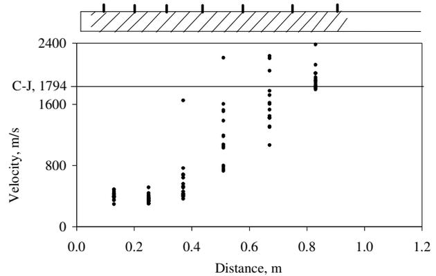
**Figure 8. Detonation-ignited thrust tube and corresponding wave speeds.**
