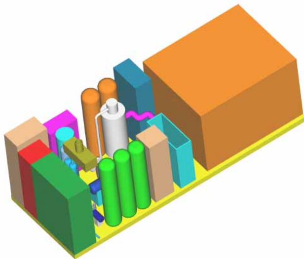
Figure 8. 625 kW Module Internal Arrangement All equipment is skid-mounted
