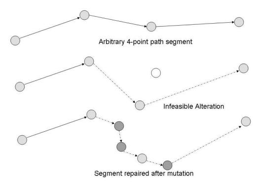
Figure 3.8 Mutate Alter Operation with Repair.
