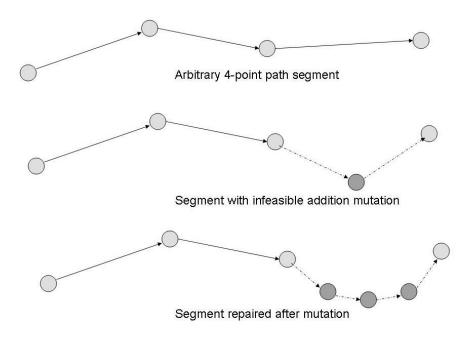
Figure 3.6 Mutate Add Operation with Repair.
