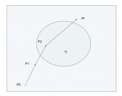
Figure 3.1 Example of Route Intersecting a Detection zone.
