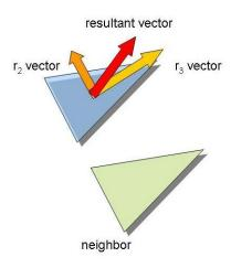
Figure 3.12 Separation Rule Applied to Swarm Member.
