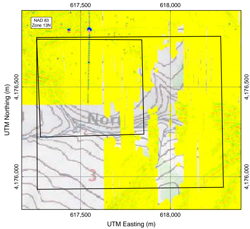
Fig. 25 – Helicopter magnetometry anomaly image of the suspected 75mm range
