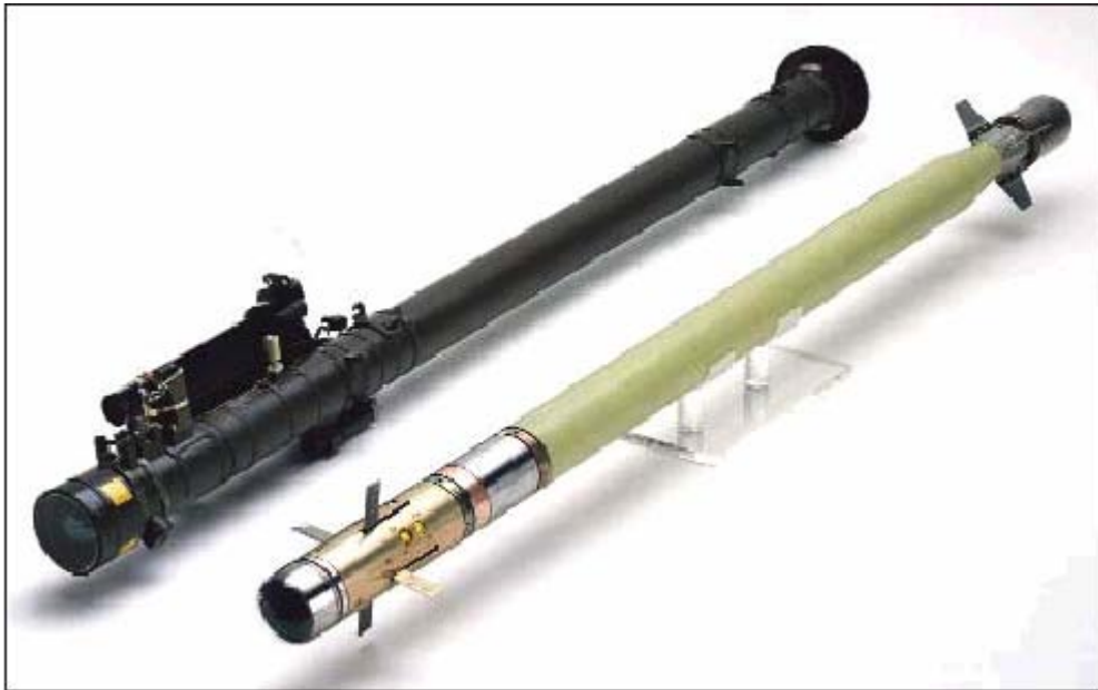
Figure 1. Stinger launch tube assembly (left) and Stinger missile round. 14
