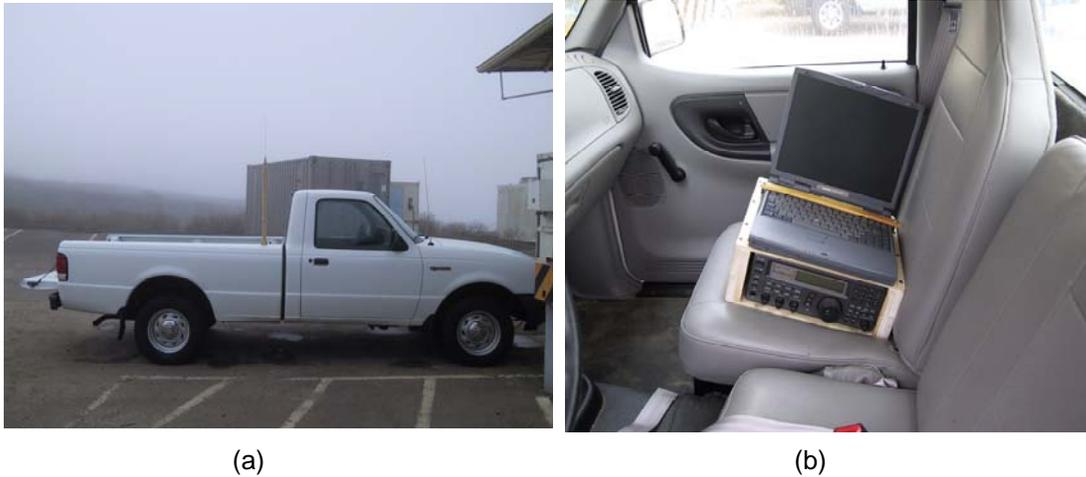
Figure 1. The receiver antenna mounted on a pickup truck (a) and the receiver with laptop computer in the truck (b).
