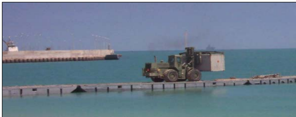
Figure 26. Rough-Terrain Cargo Handler moving container along floating causeway as part of JLOTS operation
