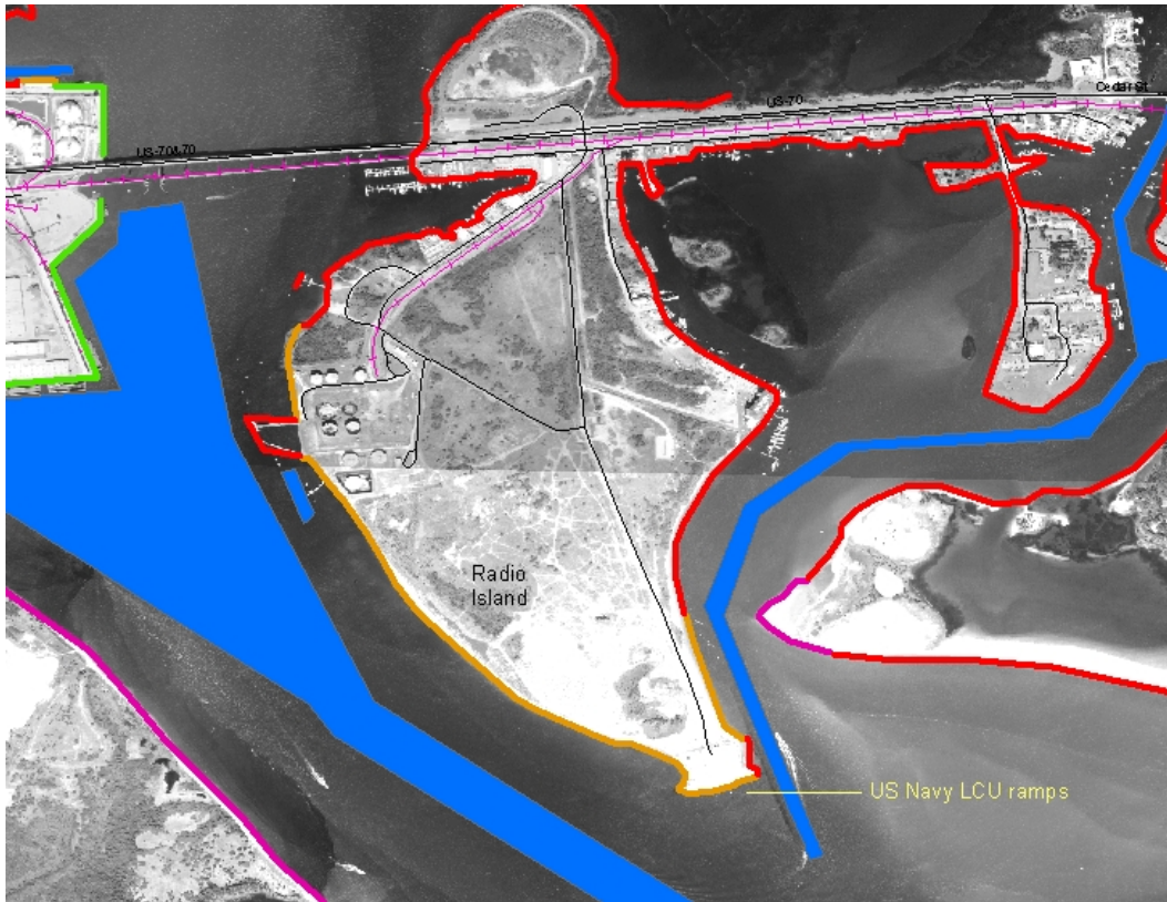
Figure 21. State Ports of North Carolina and U.S. Navy occupy Radio Island, located between Morehead City and Beaufort. The Navy's LCU ramps are at south end of island. Most of channel leading to Beaufort is less than 4.6 m (15 ft) deep, but an area just north of ramps may be suitable for causeway offloading
