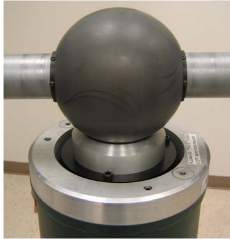
Figure 3. Space Electronics, Inc. Model SE9791 Tri-axis Spherical Air Bearing □
