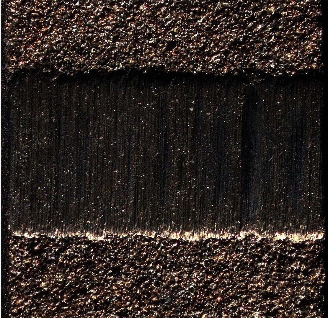
**Figure A3.1 Scar with Complete Coating Wear (Test #8)**
