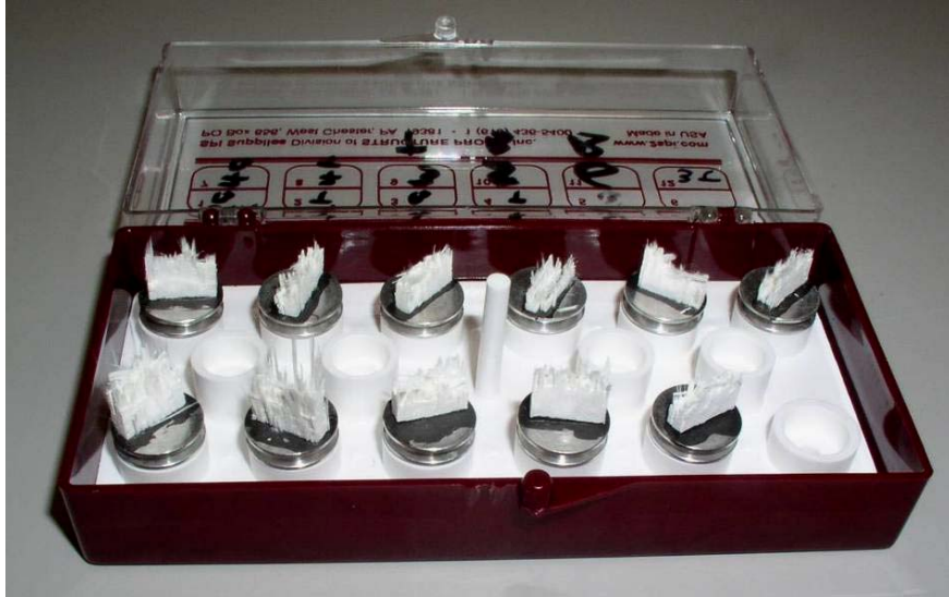
Figure 14. Uncoated N720/A specimens prepared for SEM observation.
