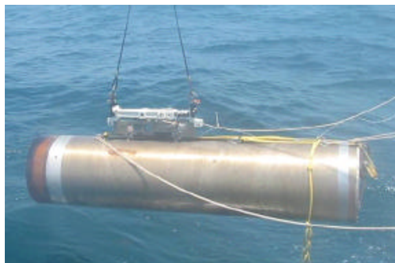
Fig. 3. Instrumented cylinder with the blunt nose attached, before an air release
