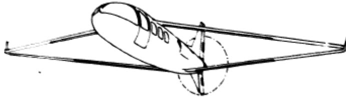
Figure 4 Positive stagger configuration with wings connected to each other [21].
