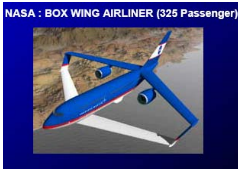
Figure 3 Negative stagger configuration using wing connectors [1].
