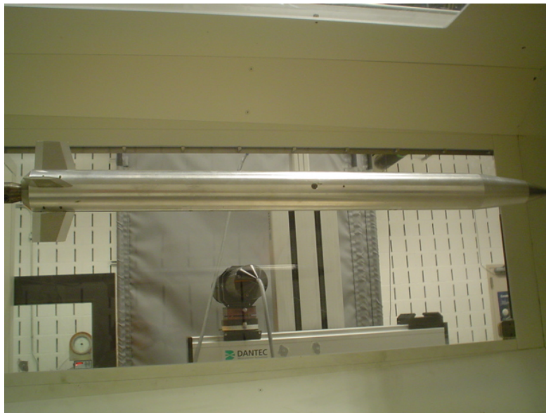
Figure 12 Bare missile model in the wind tunnel.
