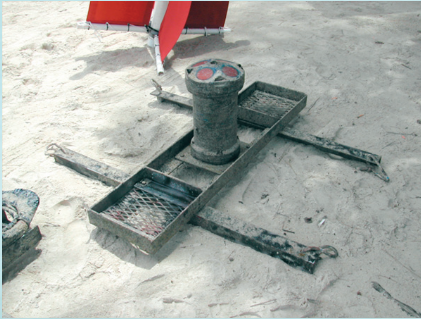
Figure 2. ADCP in frame (left) and close-up of transducer head with biofouling (right).
