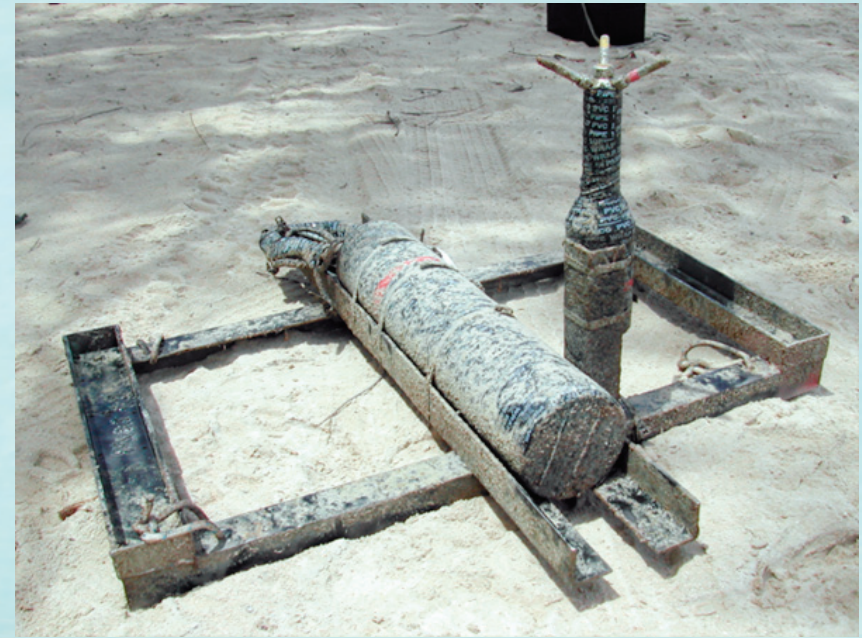
Figure 3. Hydra ADV in frame (left) and closer view of the biofouled sensor head (right).
