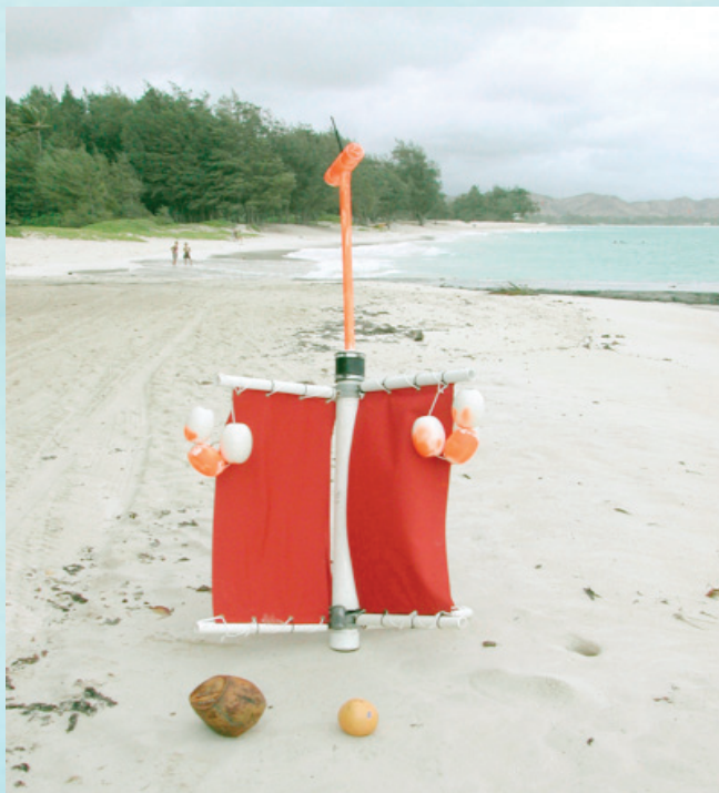
Figure 4. GPC current drogue with traditional drifter (grapefruit) and Hawaiian drifter (coconut). Drifter floats just below the surface.
