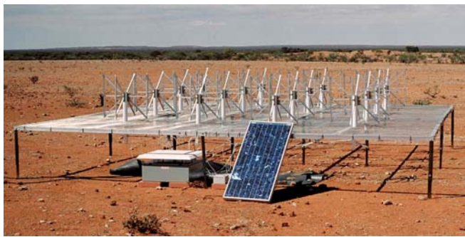
Figure 3. The first completed antenna station with beamformer box and battery-backed solar power supply.
