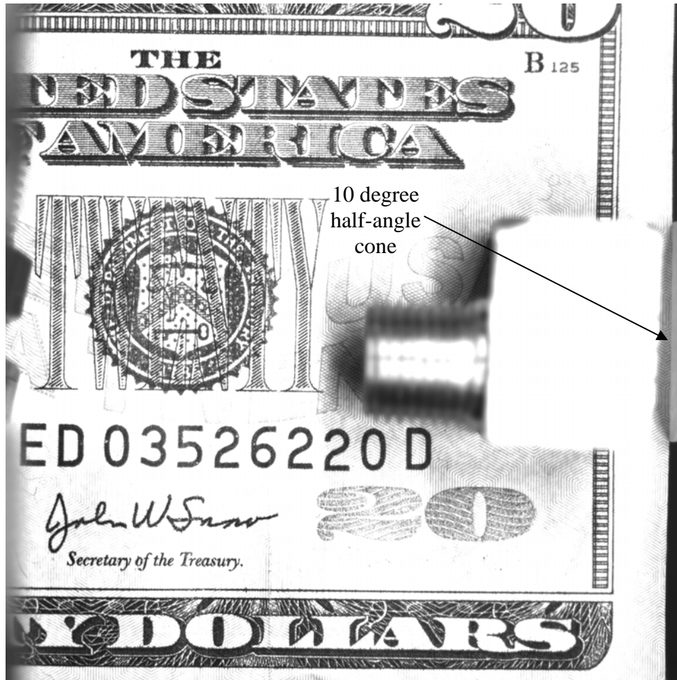
Figure 34. Sample Focusing Image : Captured with PIV camera to illustrate size of interrogation area
