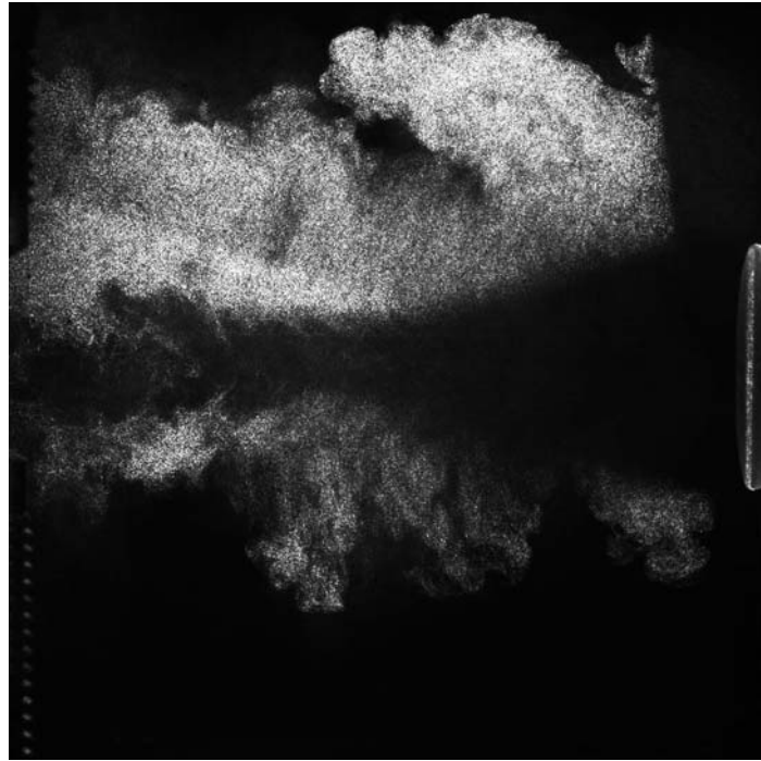
Figure 35. Nozzle Block Injection PIV Image ; 1 st Exposure, 18 \mu s delay captured with Dantec PIV system
