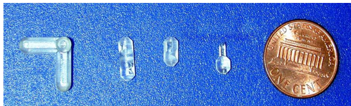
Figure 2. DSM Somos 11120 joint elements for the boom.
