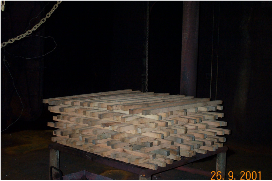
Fig. 23 — Wood crib for Comm Center
