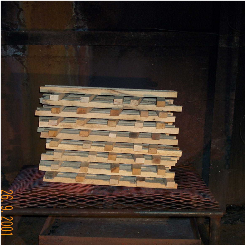
Fig. 24 — Wood crib for Radio Transmitter Room
