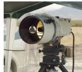
HISPEC: 8-11 micron high sensitivity single pixel fourier transform infrared spectrometer
