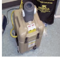
Dry Filter Unit (DFU) Biological Collector
