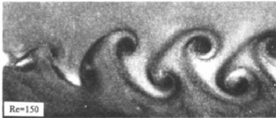
Figure 2. Development of Von Karman Vortex Streets in the Laminar Flow Regime for a Re = 150 (Williamson 2004, 480)
