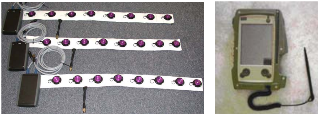
Figure A-2. Three tactile displays belt assemblies are shown above along with their tactor controller boxes (TCBs). Each box includes a wireless Bluetooth receiver and the controlling circuitry. The picture on the right is the advanced robotics controller (lightweight) PDA that remotely sends the selected signal to the TCB to trigger the tactile message.
