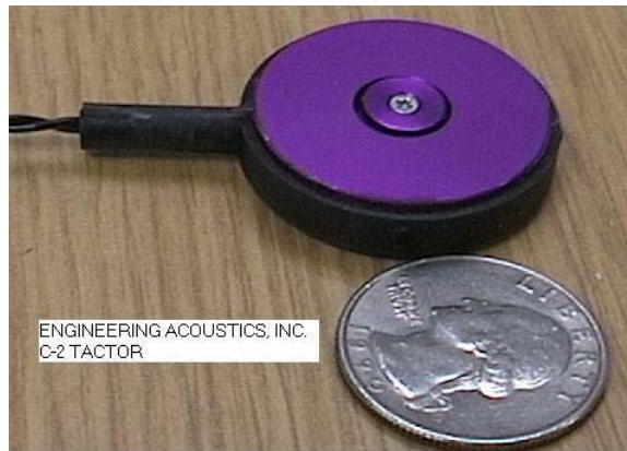
Figure A-1. Photograph of a single tactor, model C2, manufactured by Engineering Acoustics, Inc. These tactors are essentially acoustic transducers that transmit 200-300 Hz sinusoidal vibrations onto the skin. The mass of each tactor is 17 grams.
