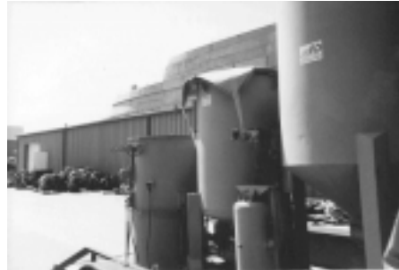
Figure 6: Abrasive Recycling Equipment Used in Demonstration
