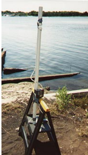
Figure 11: Typical Area Monitor Using Personal Cassettes
