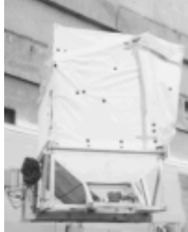
Figure 2: ARK Platform with Monarflex Material (from Field Trials - Jacksonville, FL)
