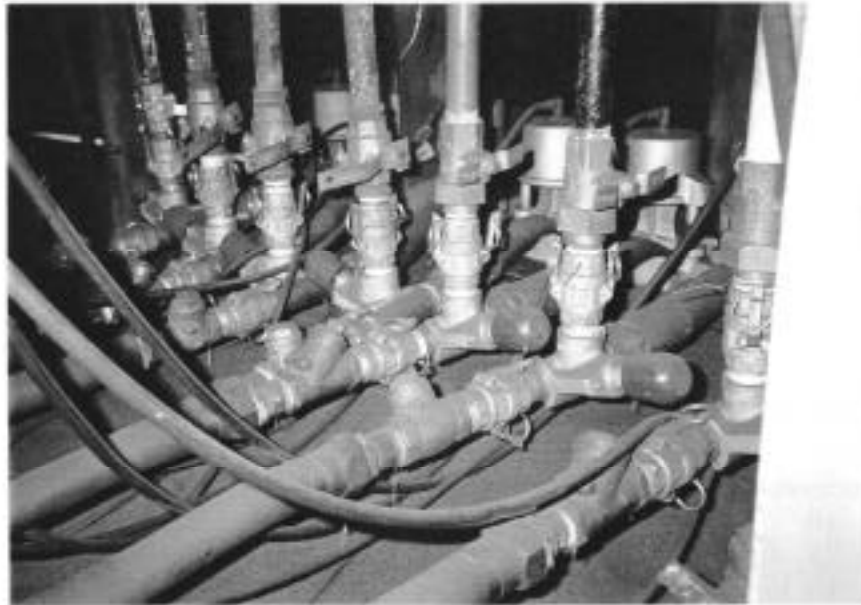
Figure 2-4 Typical Cam Lock installation on large blast pot. Note how cams are wired for safety to prevent accidental opening.
