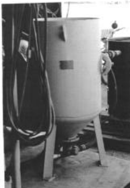
Figure 1-3: Blast Pot, 300 lb capacity, and fitted with metering valve.
