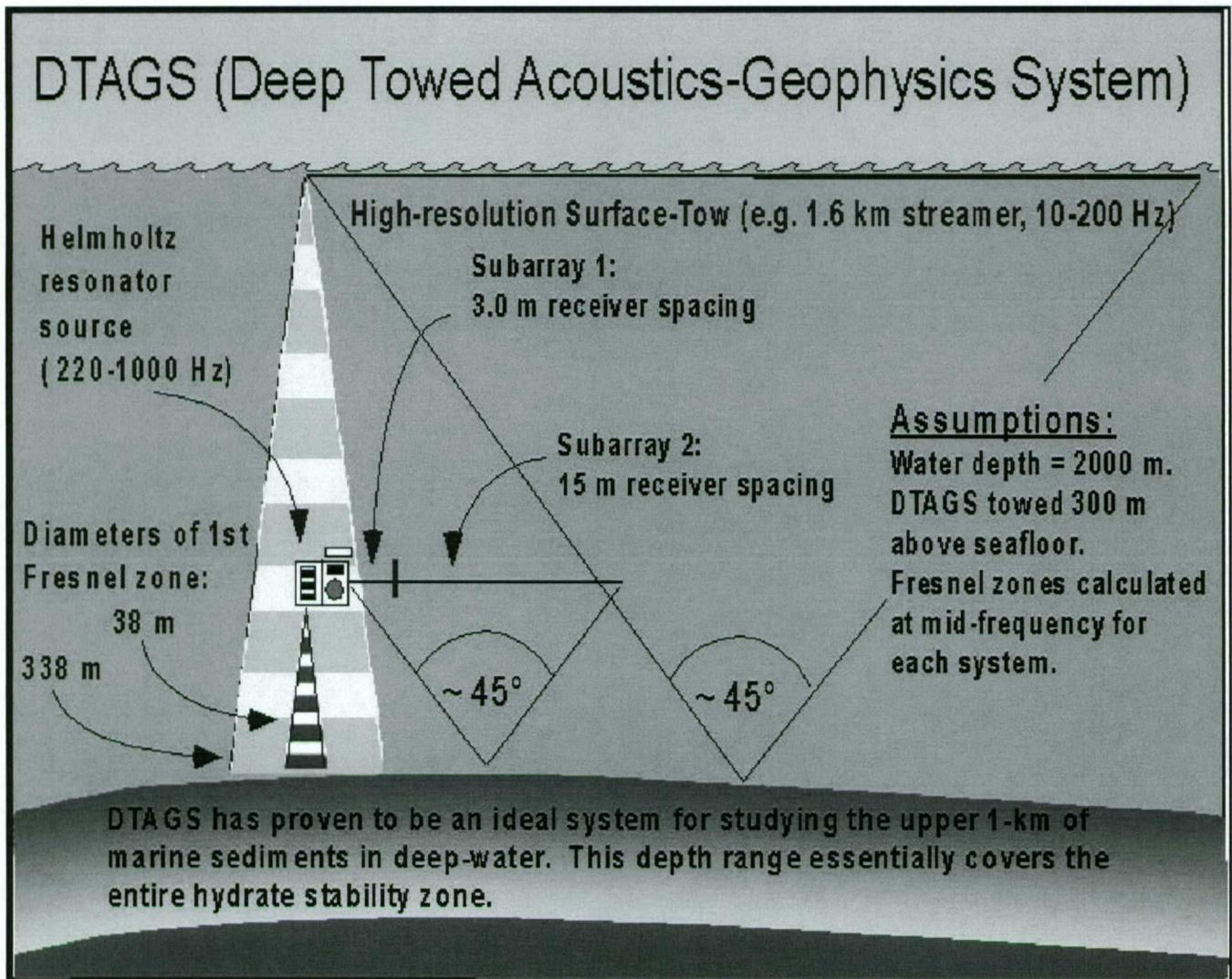
Figure 1 Cartoon demonstrating advantages of deep-tow configuration.
