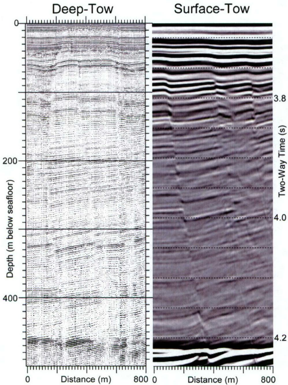
Figure 2 DTAGS data reveal details in geologic faults and structure of the BSR that is not resolved in modern surface-tow multichannel data taken on the Blake Ridge
