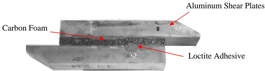
Plate Shear Specimen with Adhered Aluminum Shear Plates
