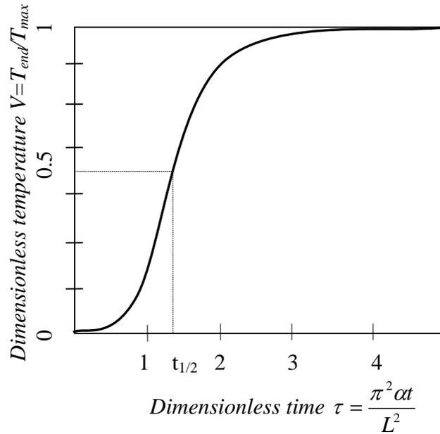
Figure 3.6.1. Dimensionless plot of rear temperature.
