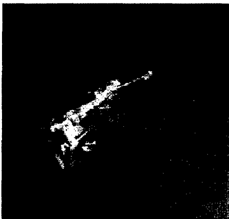
Fig. 4. SAR/IFSAR simulation and 3D model reconstruction for a backhoe simulated using SBR. (a) Simulated 2D SAR images for the backhoe target (b) 3-D SAR image for the backhoe (c) Simulated IFSAR interferogram (c) 3D model reconstructed from the IFSAR.
