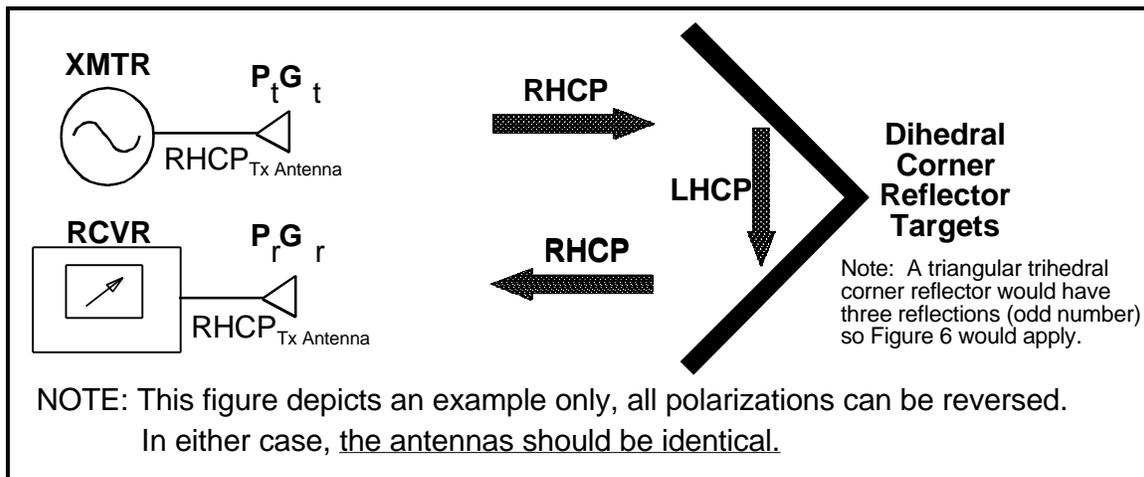
**Figure 7. Same Circular Polarization With Corner Reflector**
