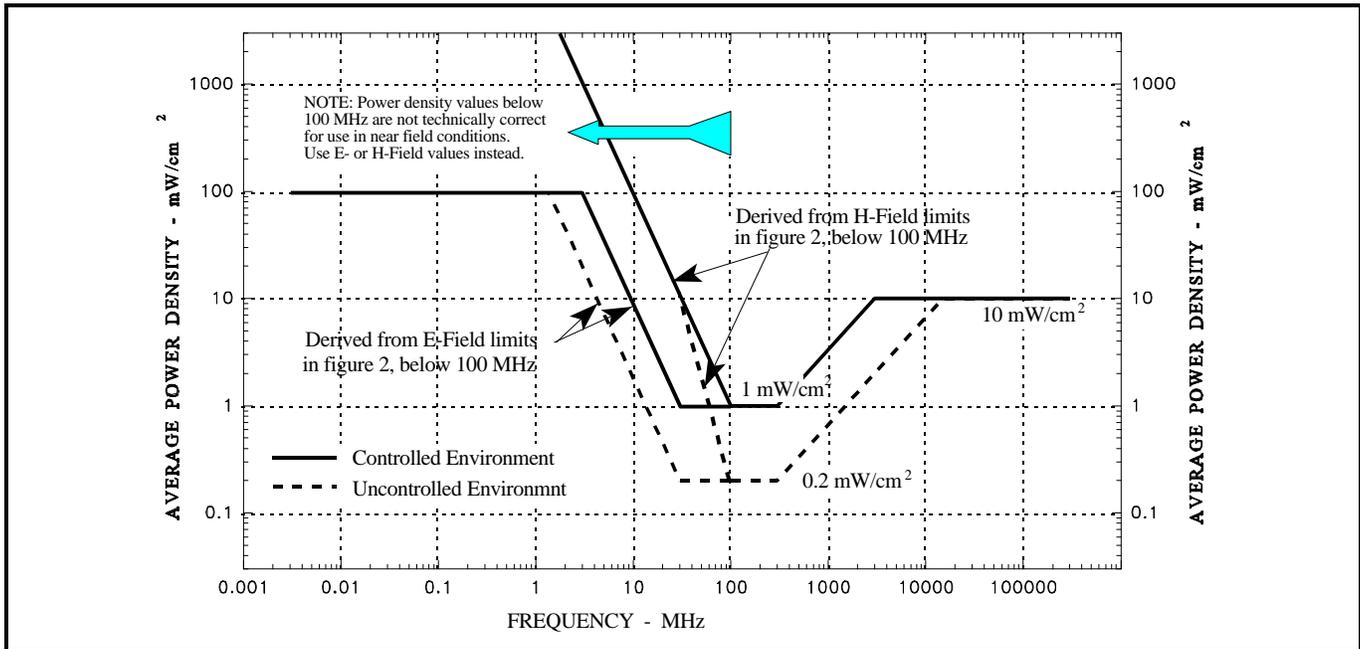
Figure 3. Radiation Hazards to Personnel from DoD INST 6055.11
