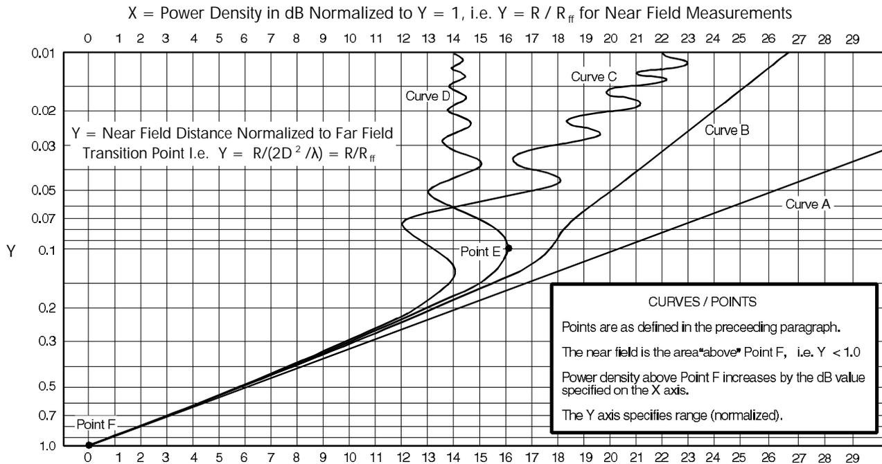
**Figure 4 - Antenna Near-Field On-Axis Power Density (Normalized)
