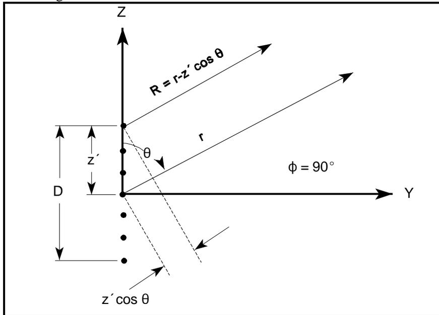
**Figure 3** - Far Field Parallel Ray Approximation for Calculations.
