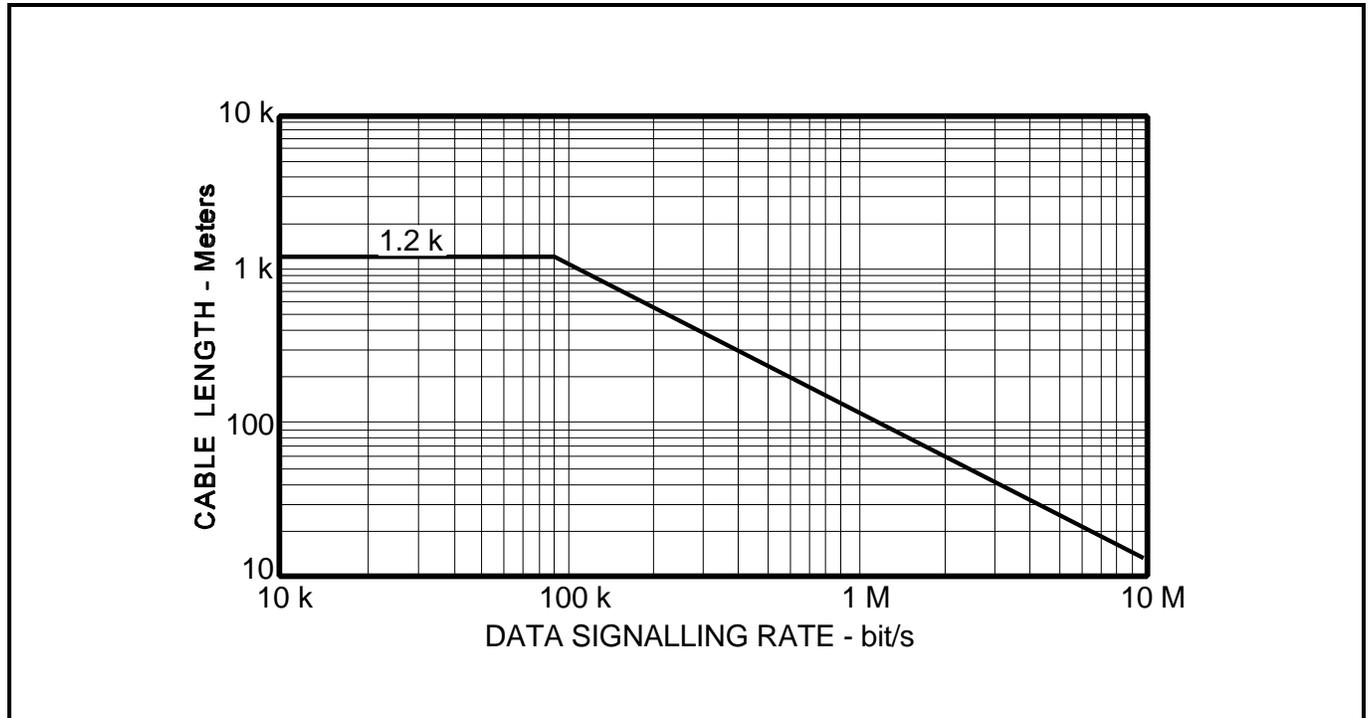
**Figure 3.** Data Signalling Rate vs Cable Length
