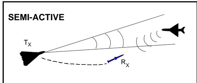
**Figure 5.** Bistatic Radar
