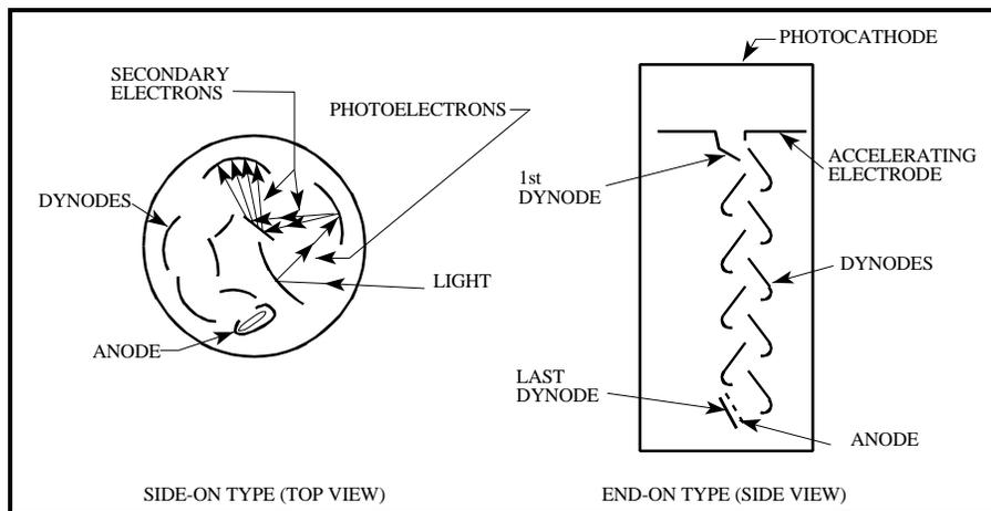
**Figure 13.** Multiplier Phototubes
