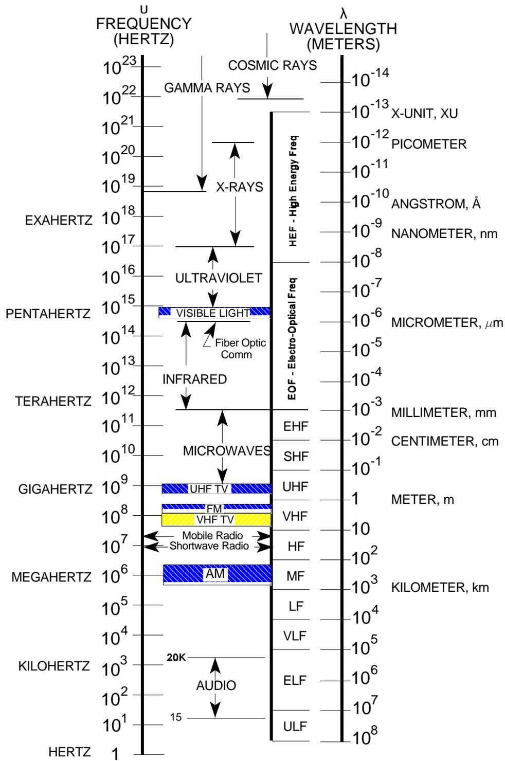
Figure 2. Electromagnetic Radiation Spectrum
