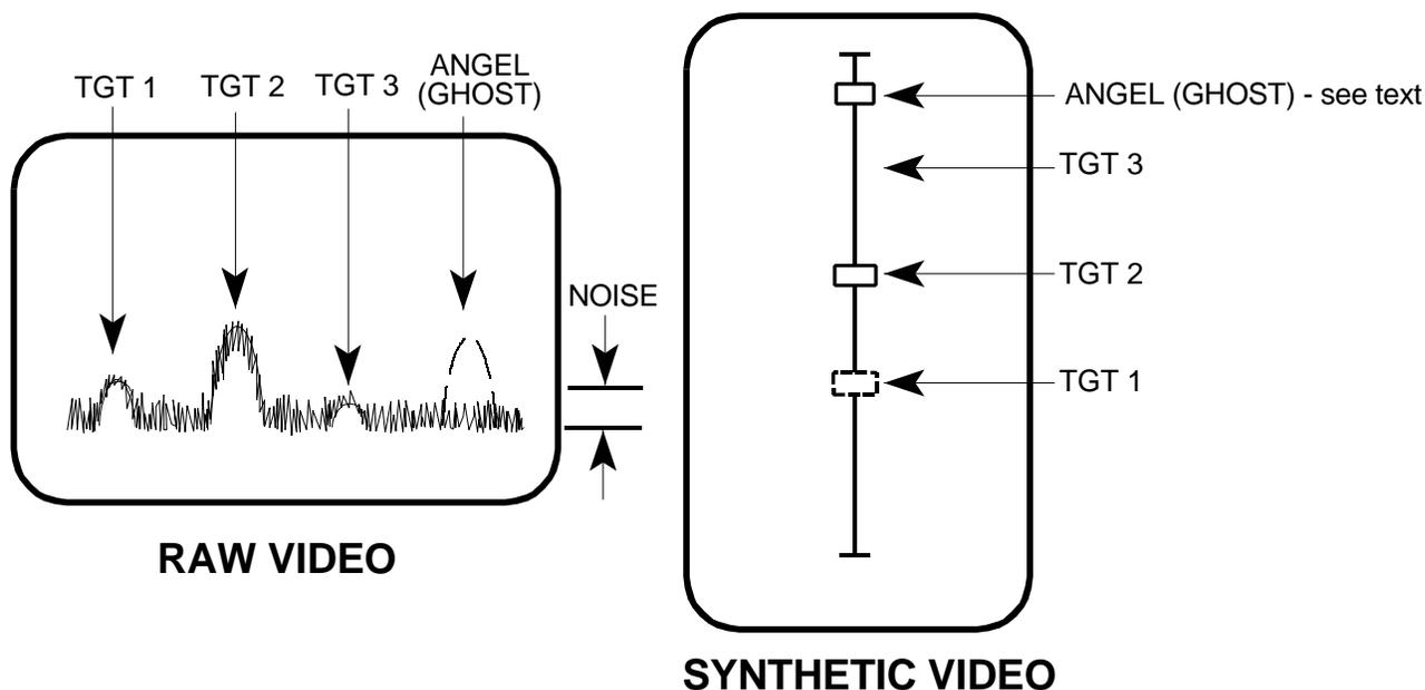
Figure 1. Radar Display Types
