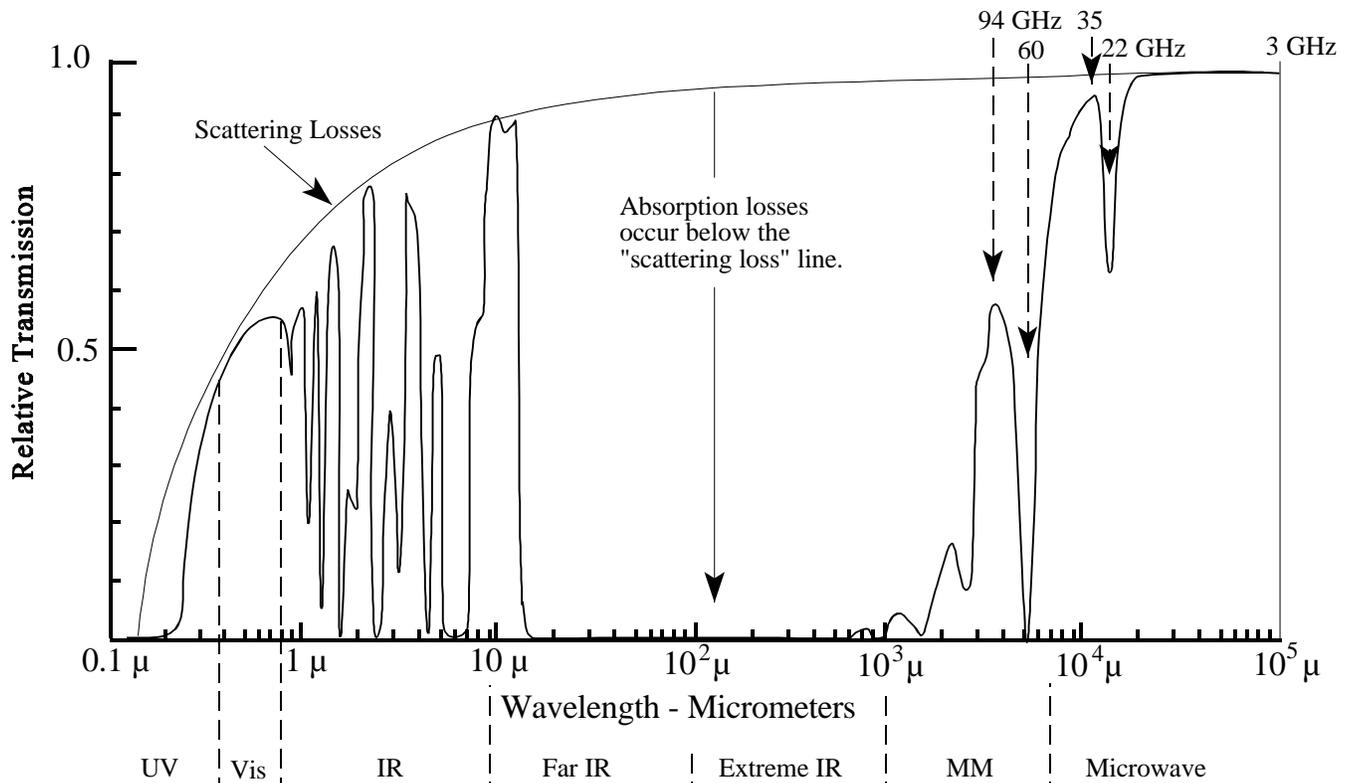
Figure 9. Atmospheric Transmission Over 1 NM Sea Level Path
