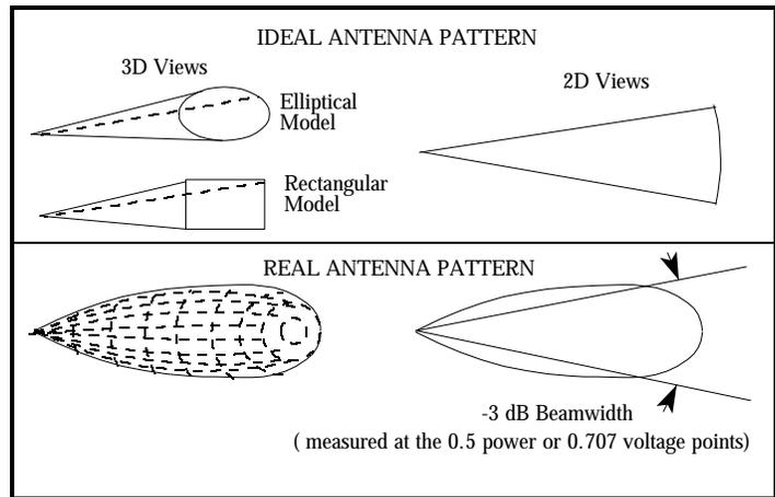
Figure 3. Antenna Beamwidth
