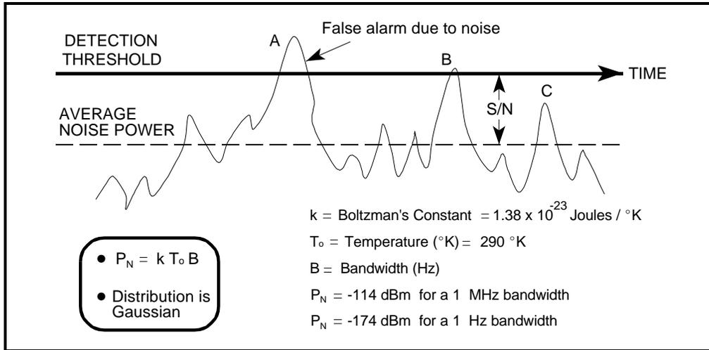
**Figure 1.** Receiver Noise Power at Room Temperature
