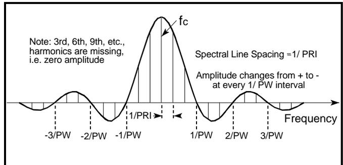
**Figure 8.** Spectral Lines for a 33.3% Duty Cycle
