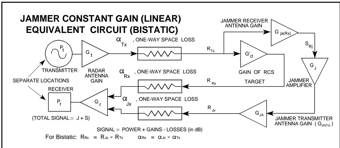
**Figure 3.** Jammer Constant Gain ECM Equivalent Circuit (Bistatic)
