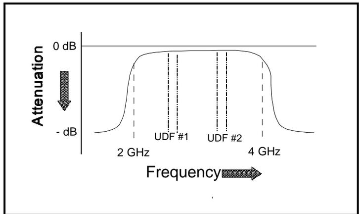
**Figure 10.** Receiver Band with Multiple UDF Entries
