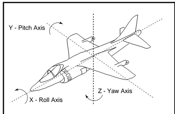
Figure 3. Reference Axes
