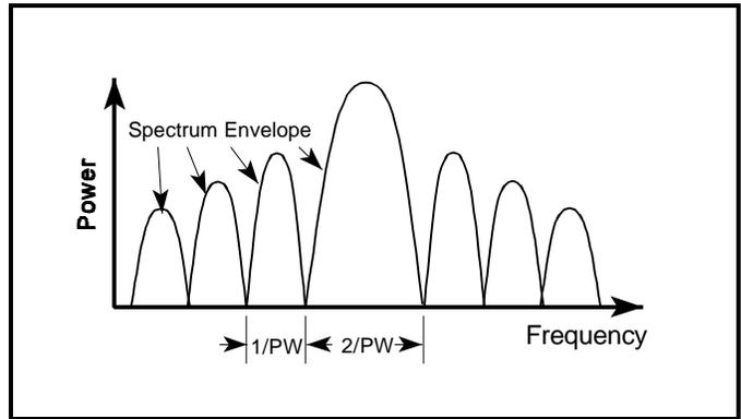
**Figure 6.** Sidelobes Generated by Pulse Modulation (Absolute Value)
