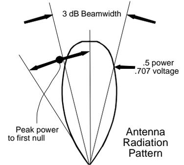
7. Parabolic Antenna Beamwidth:
