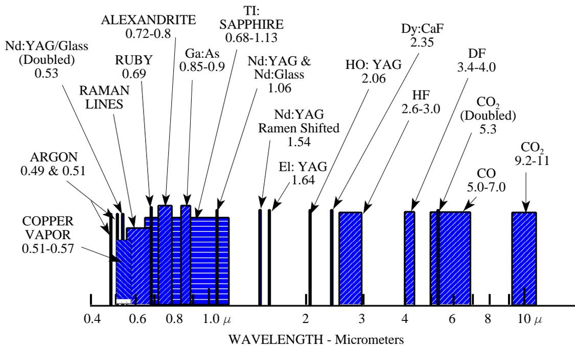
**Figure 19.** Spectral Lines / Ranges of Available Lasers
