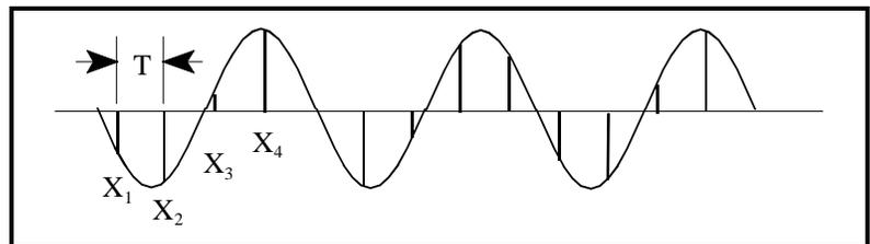
**Figure 2 Waveform Sampling**
