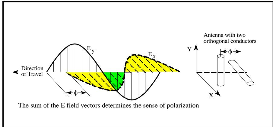
**Figure 1.** Polarization Coordinates
