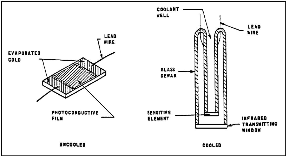
Figure 14. Photoconductive Detector
