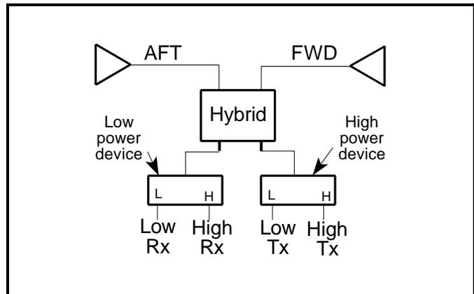
Figure 7. Alternate Low/High Band Configuration
