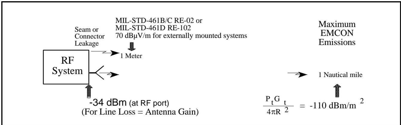
**Figure 1.** EMCON Field Intensity / Power Density Measurements
