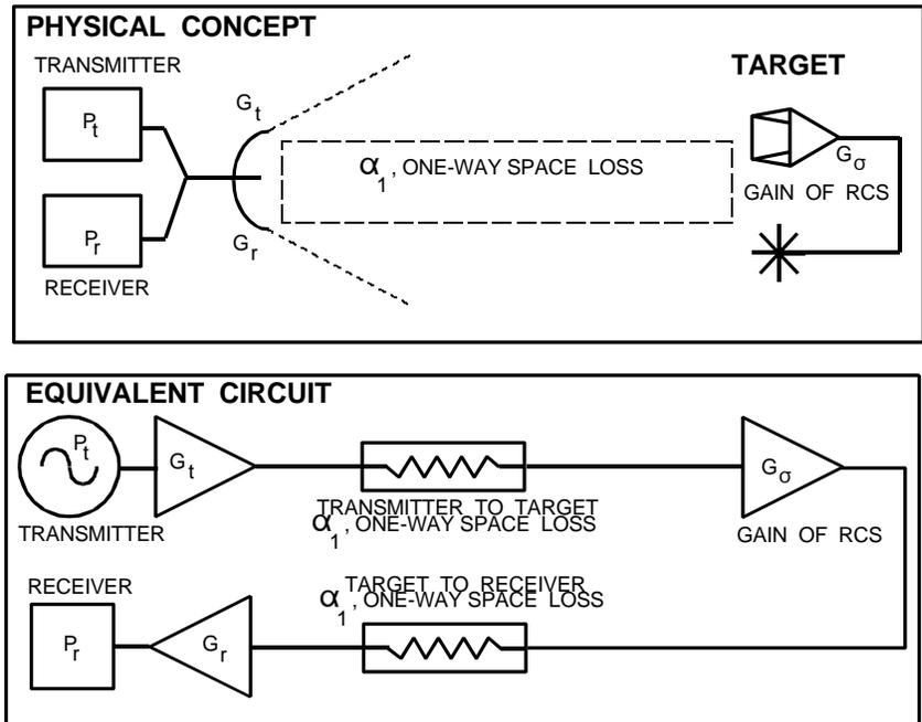
**Figure 1.** The Two-Way Monostatic Radar Equation Visualized
