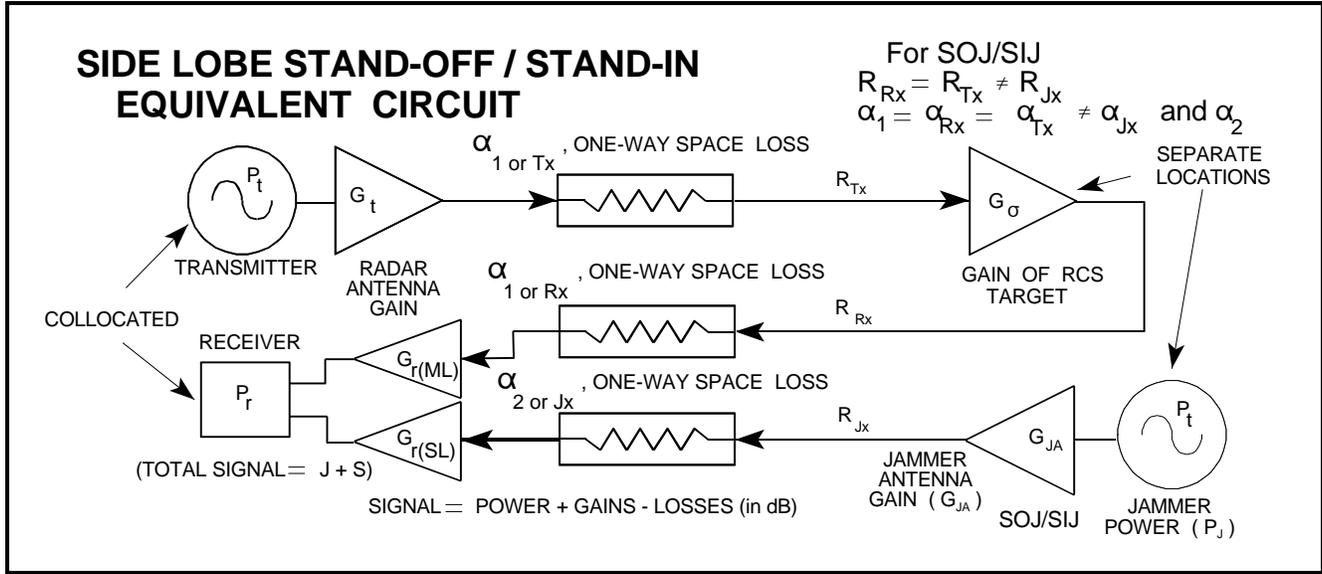
**Figure 4.** Side Lobe Stand-Off / Stand-In ECM Equivalent Circuit
