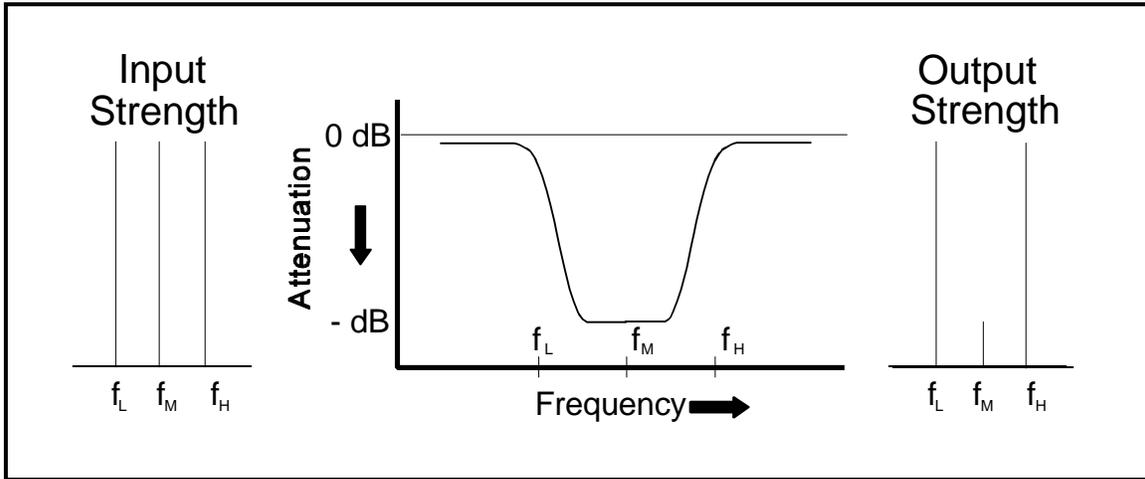
**Figure 4.** Band-Reject Filter
