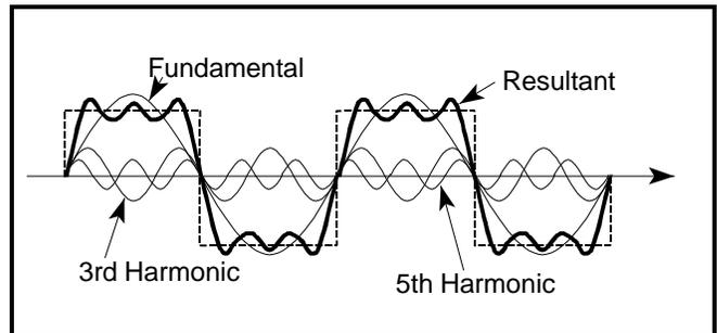
**Figure 9.** Square Wave Consisting of Sinewave Harmonics
