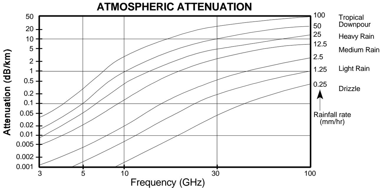
**Figure 2.** Atmospheric Attenuation
