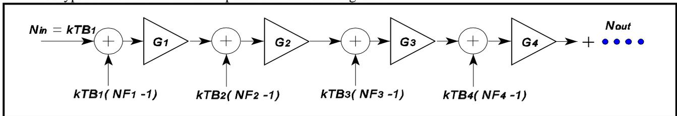
**Figure 3.** Noise Factors for Cascaded Amplifiers (NF<sub>CA</sub>)
