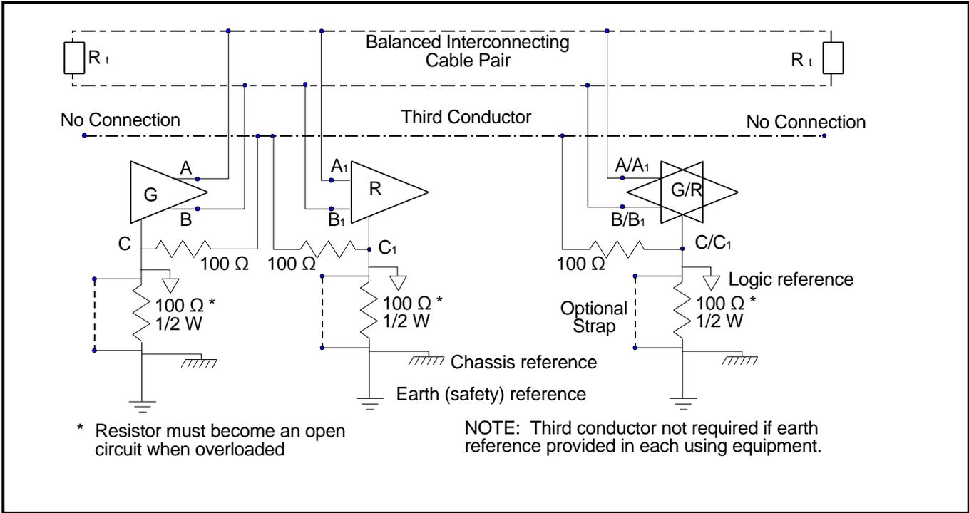
**Figure 2.** Grounding Arrangements
