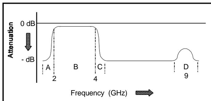
Figure 3. Frequency Areas in a Sample 2-4 GHz Receiver
