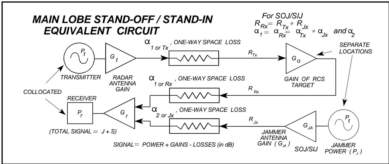
Figure 3. Main Lobe Stand-Off / Stand-In ECM Equivalent Circuit
