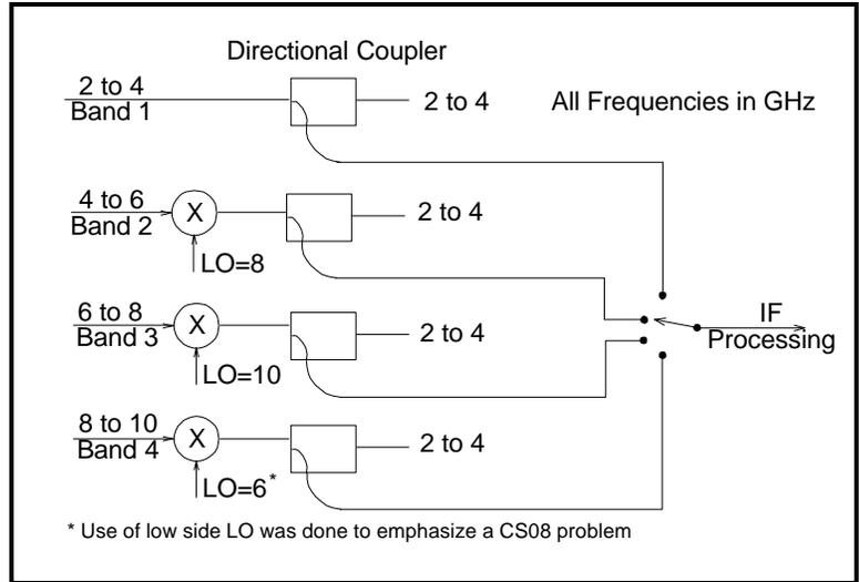
**Figure 9.** Multi Band Receiver with Common IF
