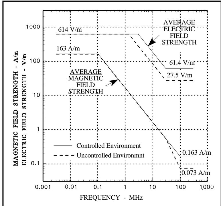
Figure 2. Lower Frequency HERP from DoD INST 6055.11
