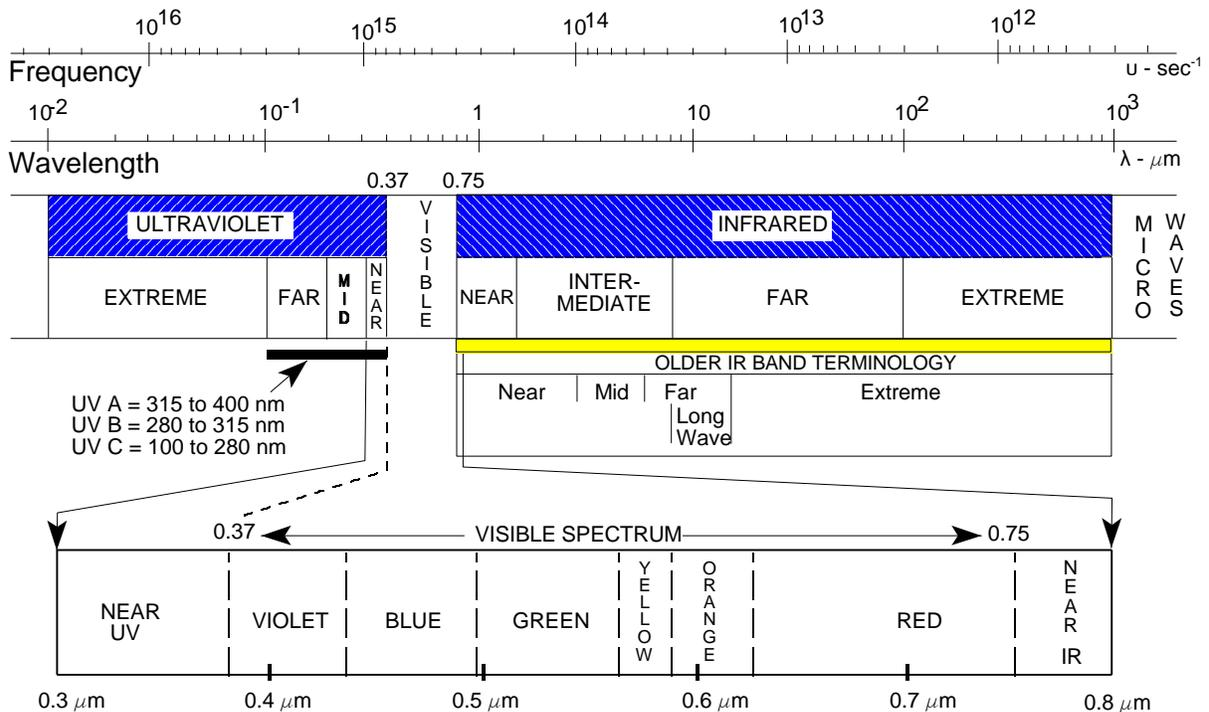
**Figure 1. Optical Spectrum**
