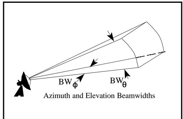
**Figure 1.** Antenna Aperture
