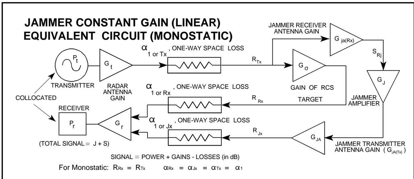
Figure 2. Jammer Constant Gain ECM Equivalent Circuit (Monostatic)
