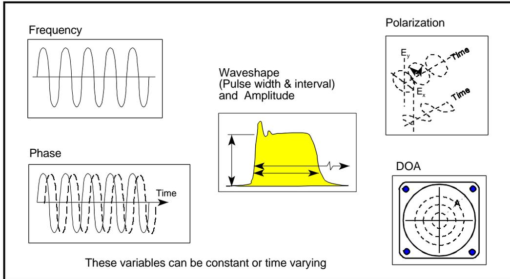
**Figure 2.** Information Content of an Electromagnetic Wave
