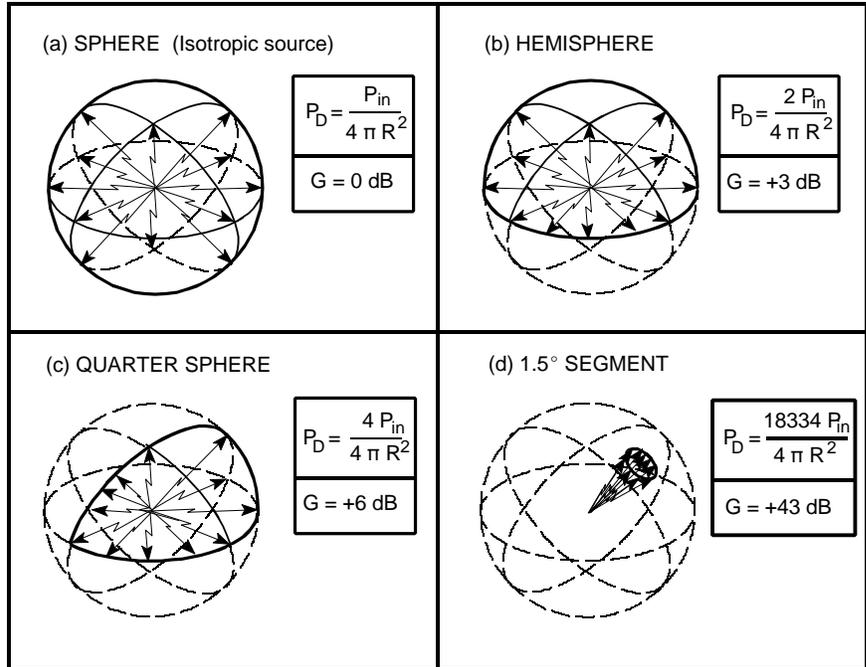
Figure 2. Antenna Gain
