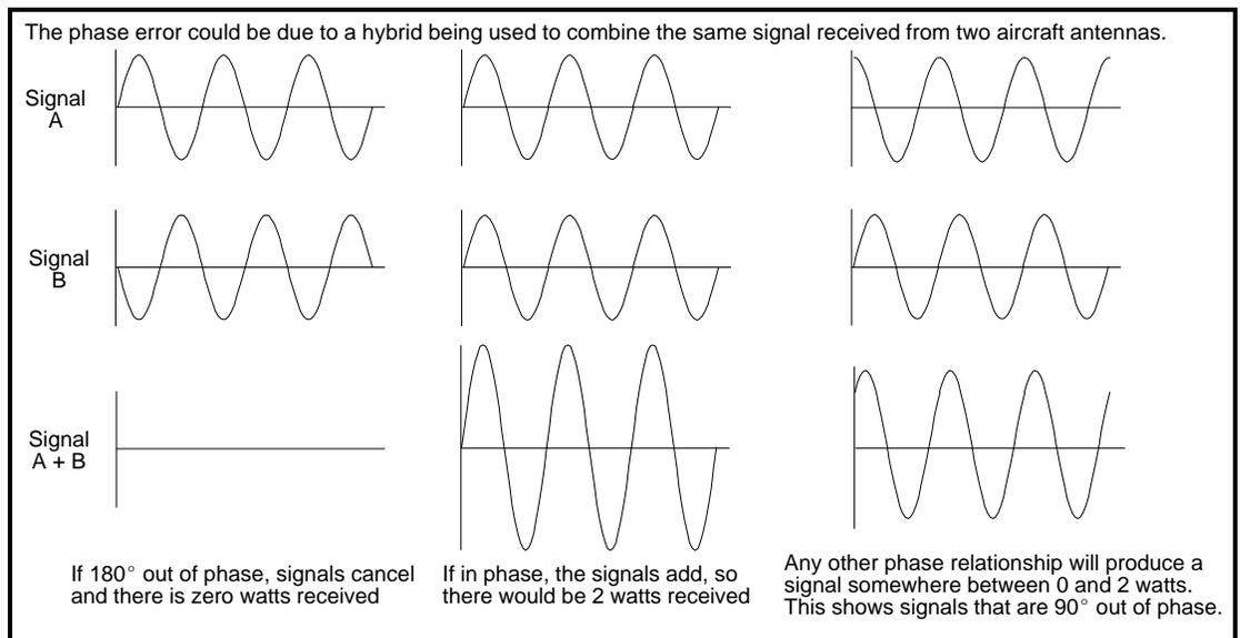
**Figure 7.** Sinewaves Combined Using Various Phase Relationships
