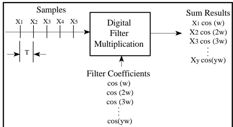
**Figure 3. Digital Filtering**
