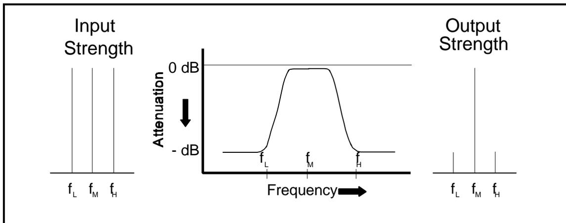
**Figure 3.** Band-Pass Filter
