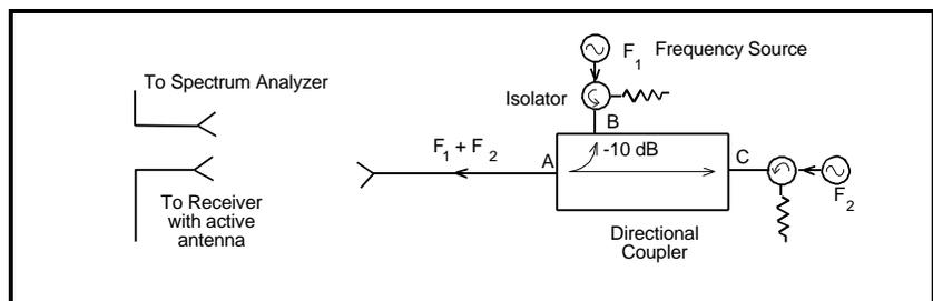
**Figure 2.** Receiver Test Setup When Antenna Is Active
