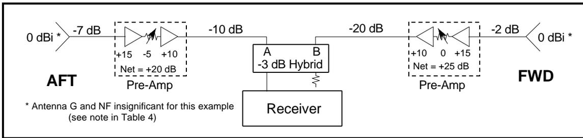
**Figure 5.** Example of Pre-Amplifier Affecting Overall Gain/Sensitivity
