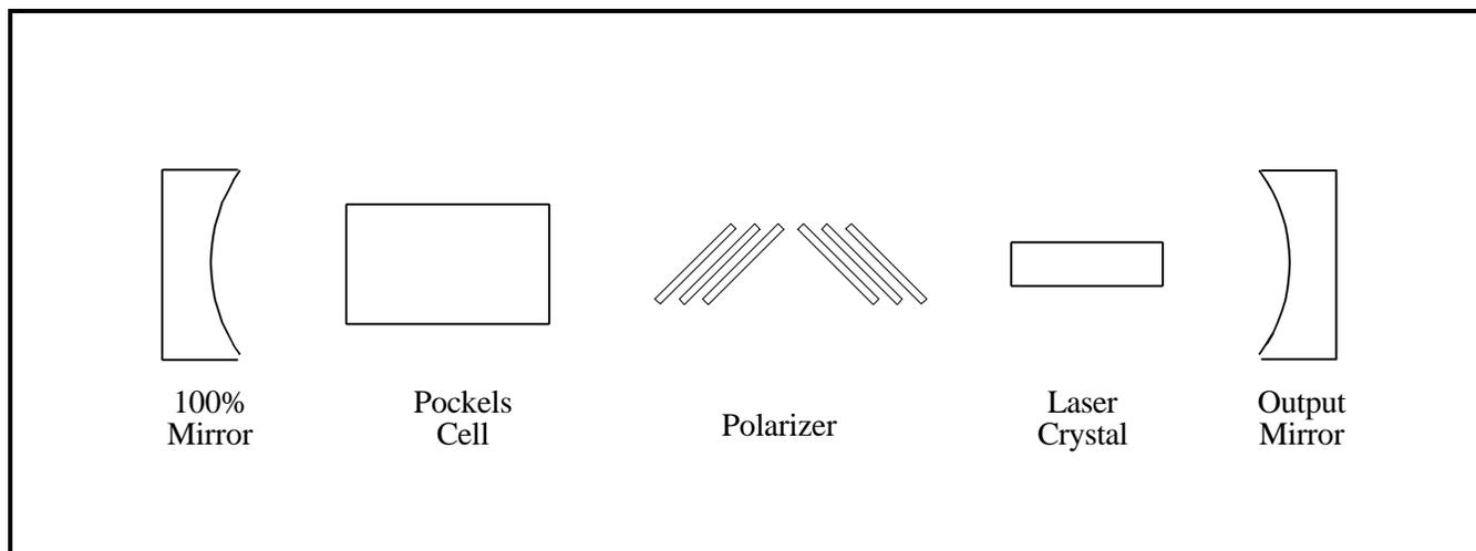
**Figure 24.** Q-switch Arrangement
