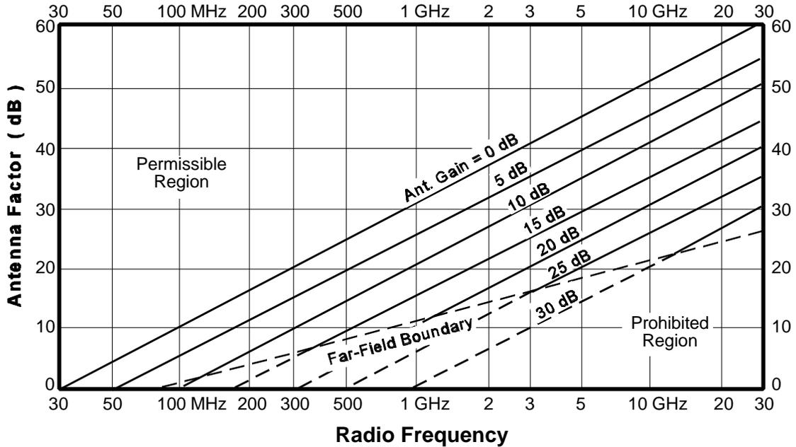
**Figure 3.** Antenna Factor vs Frequency for Indicated Antenna Gain
