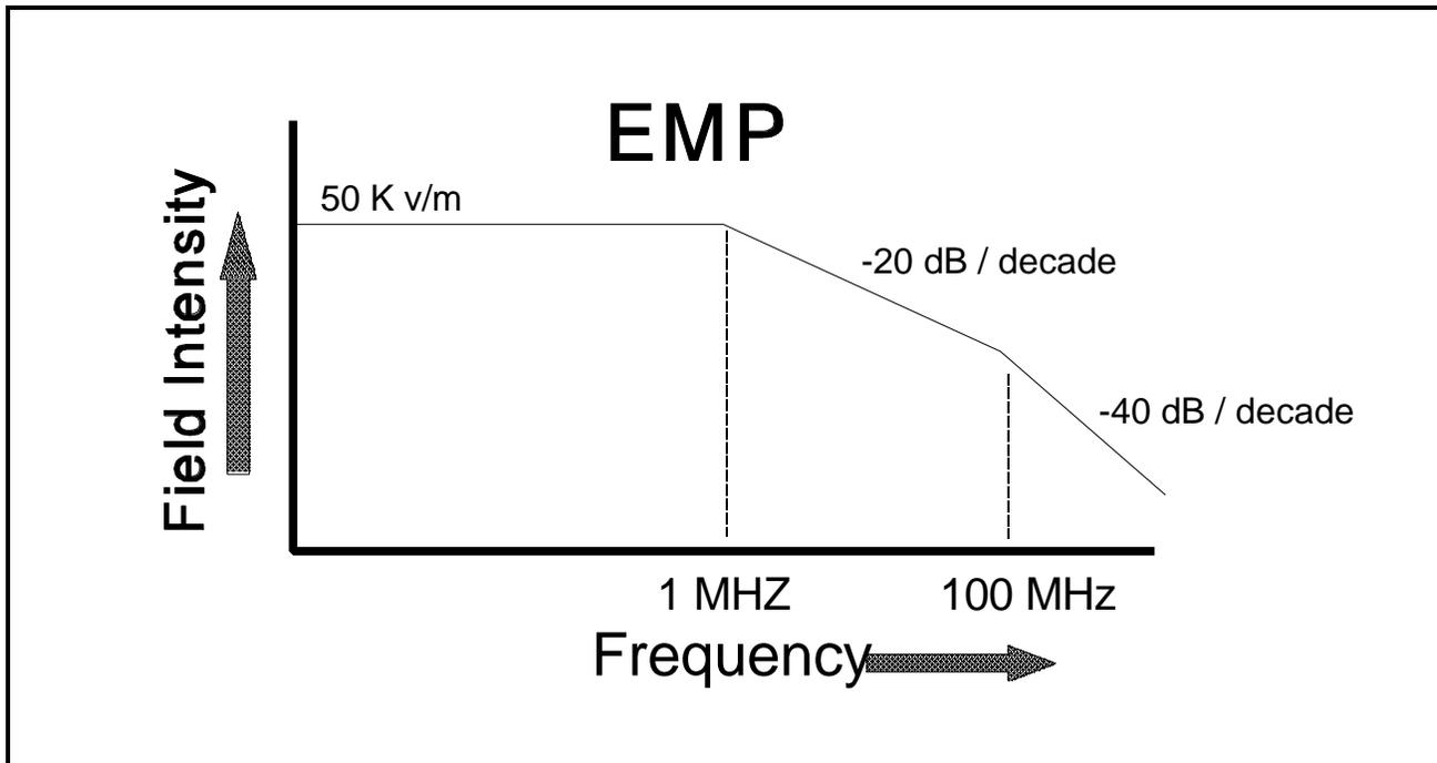
**Figure 1.** EMP as a Function of Frequency
