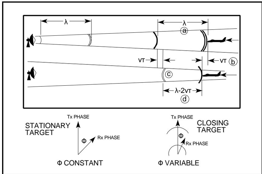
Figure 3. Doppler Compression Equivalent to Variable Phase Shift
