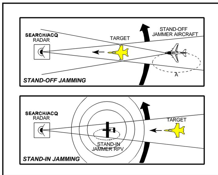
Figure 2. Support Jamming
