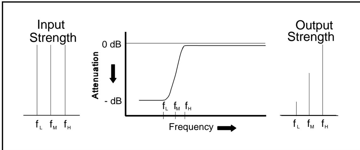
**Figure 2.** High-Pass Filter
