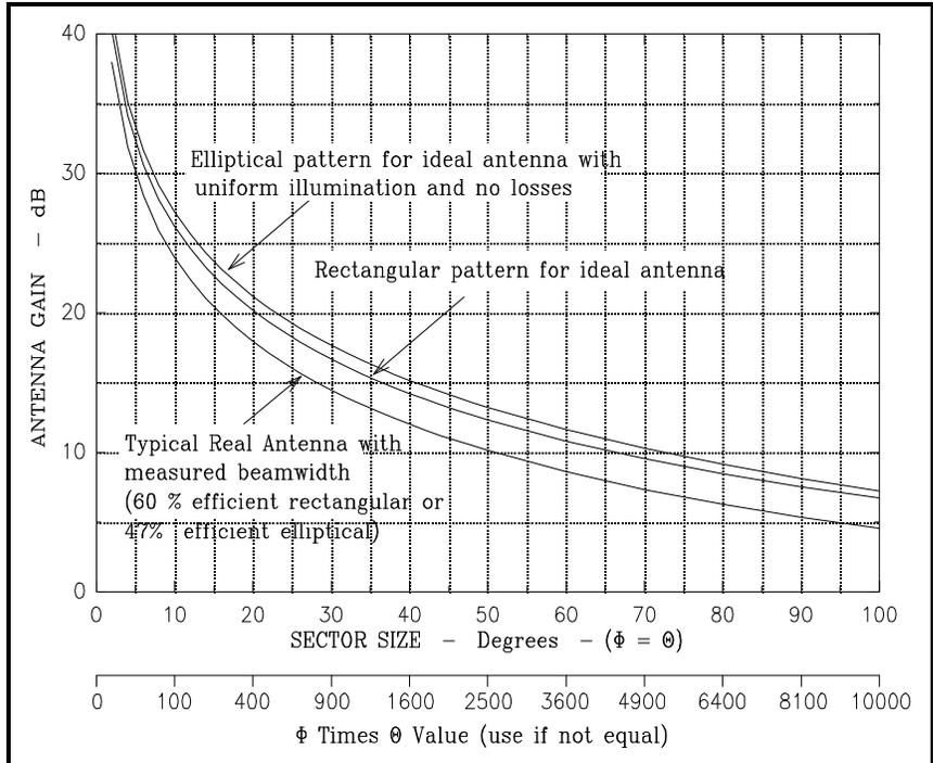
Figure 4. . Antenna Sector Size vs Gain
