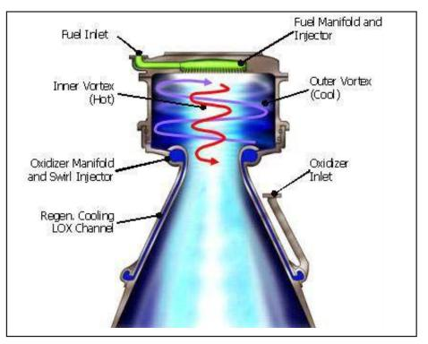
The vortex cooled chamber wall engine contains two co-axial vortices. The oxidizer flowing up from the base forms the outer, insulating vortex, and then spirals in at the head end to form the second vortex that descends to flow out of the engine nozzle. Fuel is injected at the top of this inner combustion vortex. (Source: Orbital Technologies Corporation (ORBITEC<sup>TM</sup>))
