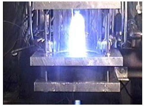
**ABOVE:** Oxygen and hydrogen burn in a VCCW chamber. The combustion chamber, constructed of Plexiglas, demonstrates the vortex cooled chamber wall concept. The Plexiglas walls remain cool and undamaged even though the temperature in the core vortex is 3000 C. (Source: Orbital Technologies Corporation (ORBITEC<sup>™</sup>)) **BELOW:** Aquarius Mission Profile. Low cost launch is achieved through relaxed reliability. (Source: Space Systems/Loral)
