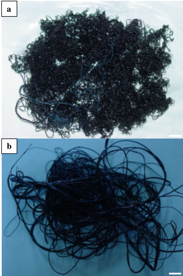
Figure 2. Digital photographs of as-spun single fibers from (a) MWNT-g-pPEK and (b) VGCNF-g-pPEK in PPA/P 2 O 5 dopes. Scales bars are 1 cm.
