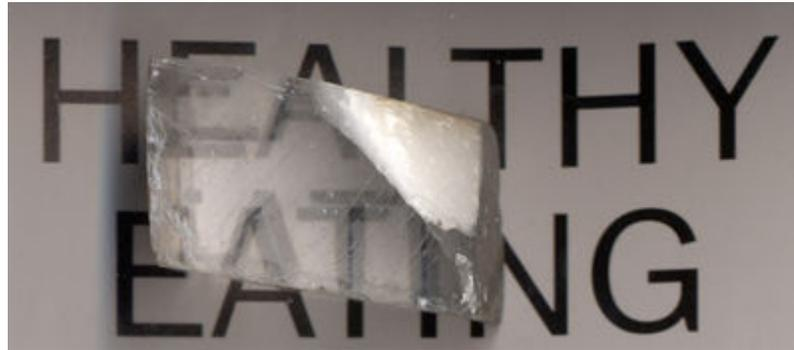
Figure 49 Birefringent Material: A calcite crystal laid upon a paper with some letters showing the double refraction
