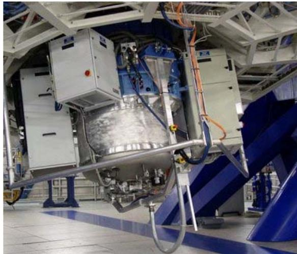
Figure 32 The SINFONI Adaptive Optics Package<sup>40</sup>
