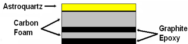
Figure 1.1 CLAS Material Typical Cross Section
