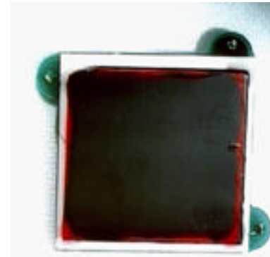
Figure 1. Finished detector 25 mm x 25 mm x 3mm mounted on PC board
