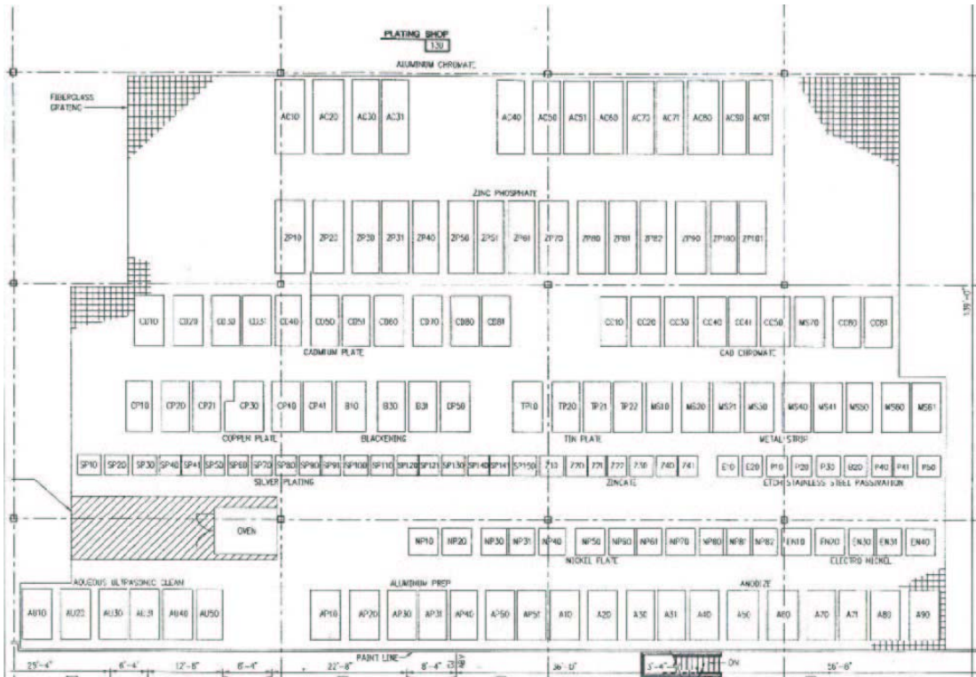
Figure 3. Plating tank layout.
