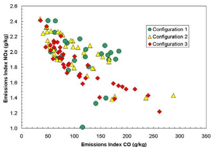
**Figure 23: NO<sub>x</sub>-CO emissions trades for the three test configurations.**
