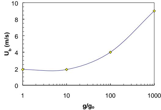
**Figure 7: Flame Speed Determined at a Height of 0.18 mm for Different Gravitational Forces.**
