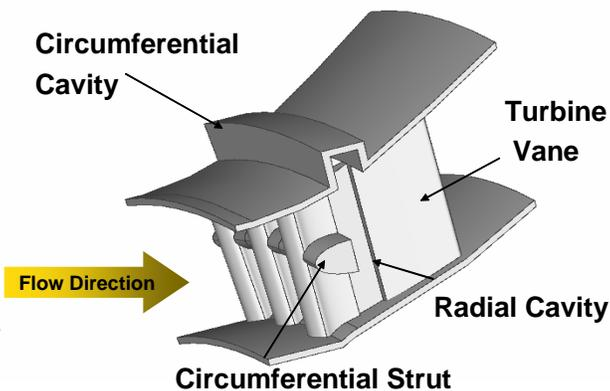
**Figure 2: Ultra-Compact Combustor Concept Showing Integral Circumferential Cavity and Turbine Vanes.**
