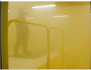
• System Testing (MOPP 4 ensembles) in aerosol chamber at Research Triangle Inc., NC.
