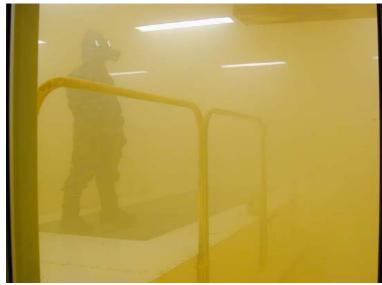
• System Testing (MOPP 4 ensembles) in aerosol chamber at Research Triangle Inc., NC.
