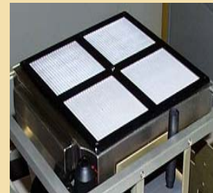
High flow (3,000+ lpm) Virtual Impactor Concentrator using a large horizontal array of mini-slits
