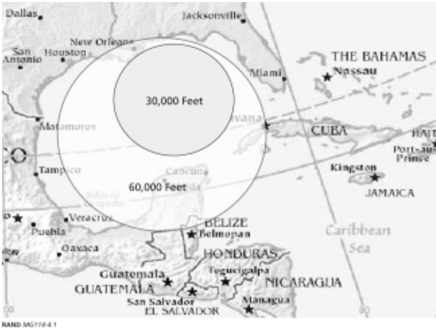
Figure 4.1 Theoretical Radar and SIGINT Coverage Area, 30,000-ft Versus 60,000-ft Altitude
