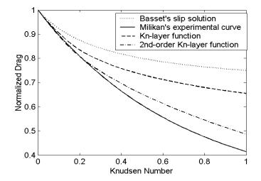
**FIGURE 5.** Normalized drag over an unconfined sphere over a range of Knudsen numbers. Experimentally-fitted curve [6] (—), Basset's slip solution [7] (···), Navier-Stokes solution with Maxwellian slip and the *Knudsen-layer wall function* (– ·). [The characteristic length used to define the Knudsen number is the sphere radius.]
