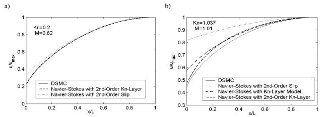
**FIGURE 4.** Normalized velocity profiles in rarefied Poiseuille flow. DSMC results (—), Navier-Stokes solution with *second-order* fictitious slip [5] (···), Navier-Stokes solution with Maxwellian slip and the *Knudsen-layer wall function* (– ·), Navier-Stokes solution with Maxwellian slip and the *second-order Knudsen-layer wall function* (– –): (a) Kn=0.2, M=0.82; (b) Kn=1.06, M=1.01.
