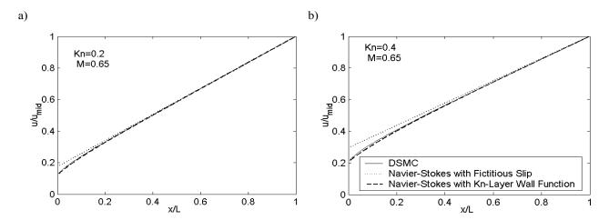
**FIGURE 2.** Normalised velocity profiles in rarefied Couette flow. DSMC results (—), Navier-Stokes solution with fictitious slip (···), Navier-Stokes solution with Maxwellian slip and the Knudsen-layer wall function (-). The wall at x/L=0 is stationary and that at x/L=2 is moving at M=0.65 with Knudsen numbers (a) Kn=0.2 and (b) Kn=0.4.
