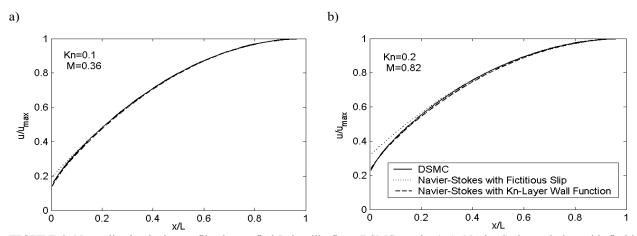
**FIGURE 3.** Normalized velocity profiles in rarefied Poiseuille flow. DSMC results (—), Navier-Stokes solution with fictitious slip (···), Navier-Stokes solution with Maxwellian slip and the Knudsen-layer wall function (– –): (a) Kn=0.1, M=0.36; (b) Kn=0.2, M=0.82.
