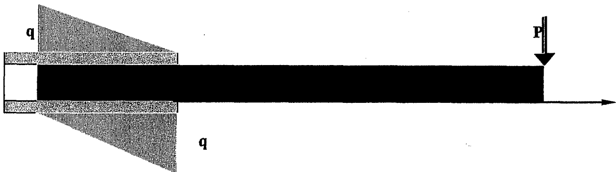
Figure 4.8 Considered Beam Distributed Loading
