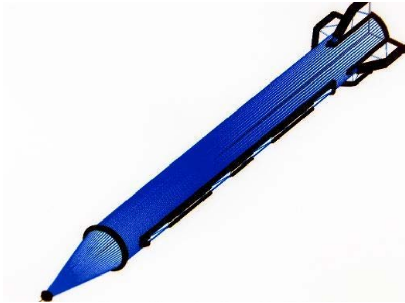
Figure 3-6: Screenshot of a missile facet file (blue) along with its corresponding extracted edges (black) viewed in XPatch.
