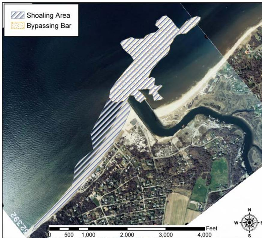
Figure 49. Delineation of shoaling area and bypassing bar
