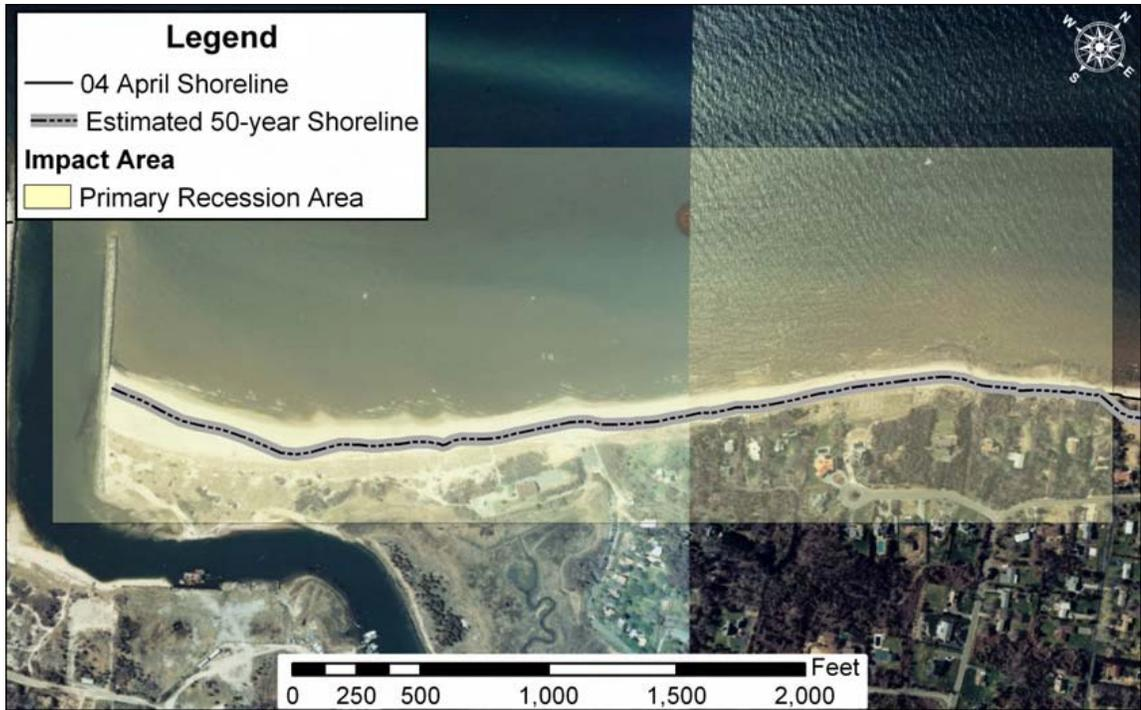
Figure 57. Extrapolated 50-year shoreline based on present conditions produces little expected change in primary erosion area
