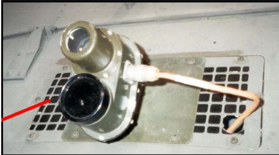
Figure 5. Universal Tracking Device mounted on a UH-60 [5]
