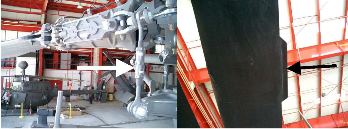
Figure 4. A PCR on a UH-60 (left) and a Trim Tab on an OH-58 [5]
