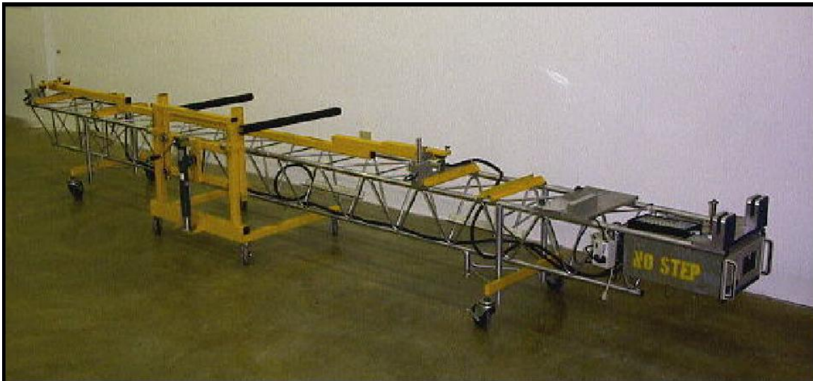
Figure 2. Universal Static Balance Fixture. This piece of equipment is utilized to statically balance the spanwise moment prior to installation [5].
