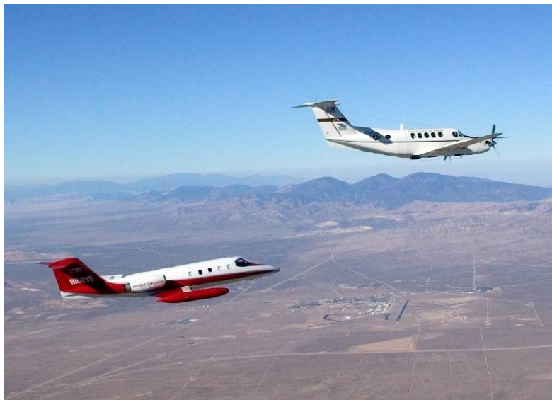
Figure 9. C-12 and Learjet in Fully Autonomous Formation Flight, Contact Position
