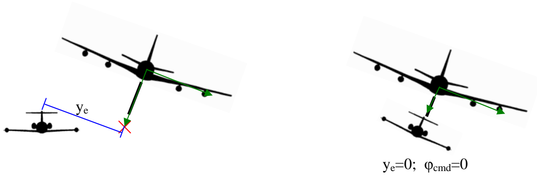
Figure 41. Requirement for Lead Bank Angle Feed Forward Control
