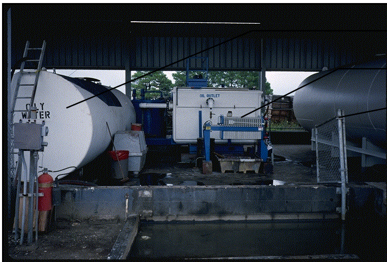
Figure 11: Oily water Separation unit - Air Dissolved Flotation
