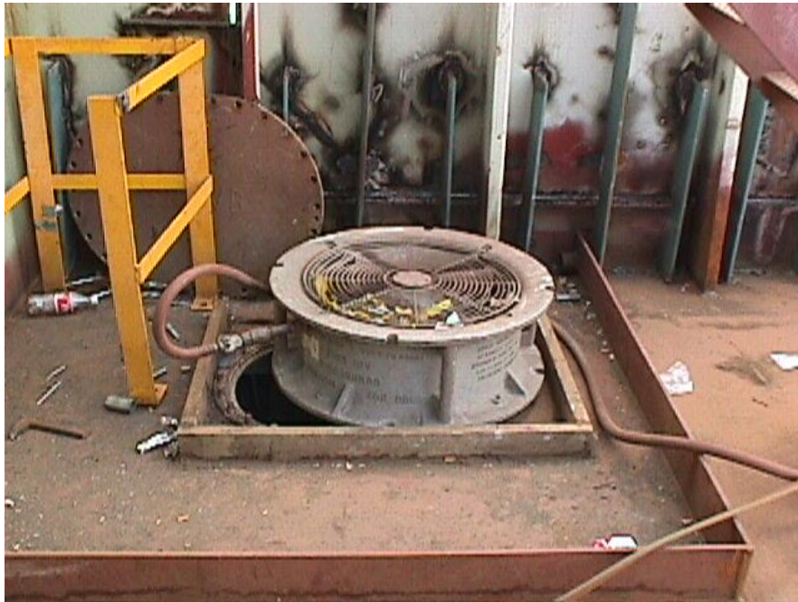
Photograph 1. Pneumatic powered portable ventilation fan propped over tank hatch cover aboard ship under construction
