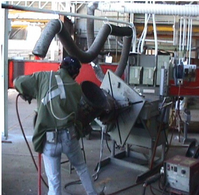
Photograph 6. Fixed fume extractor system with moveable suction hose inside fabrication shop
