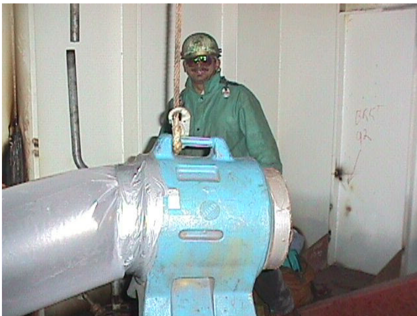
Photograph 7. Portable fume extraction fan hung from ceiling by rope during welding of bulkheads for ship construction
