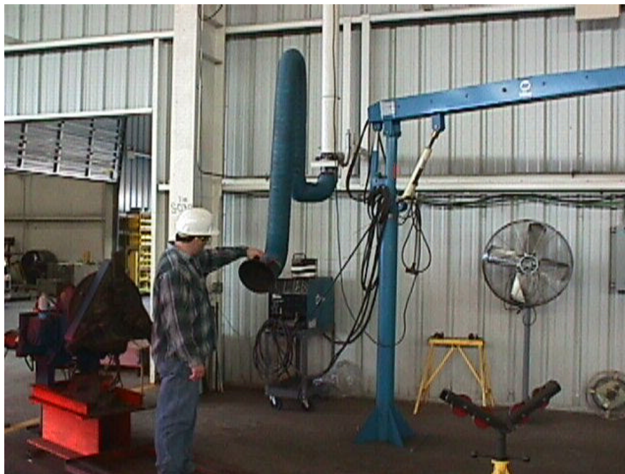
Photograph 4. Portable fume extraction hose on articulating arm for easy positioning
