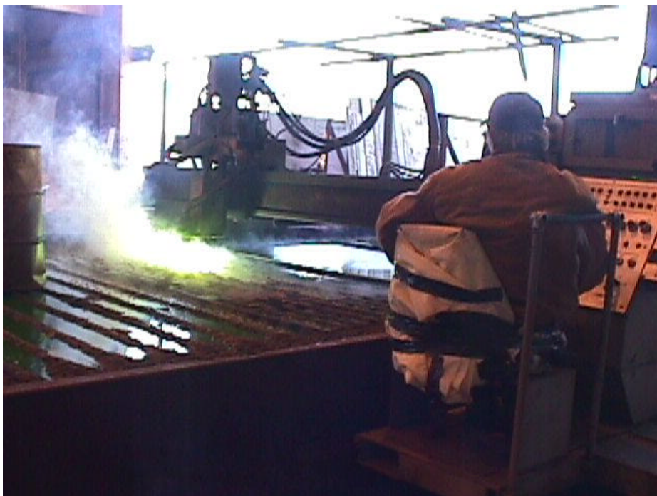
Photograph 9. Plasma cutter with no engineering controls in place to capture fumes generated.
