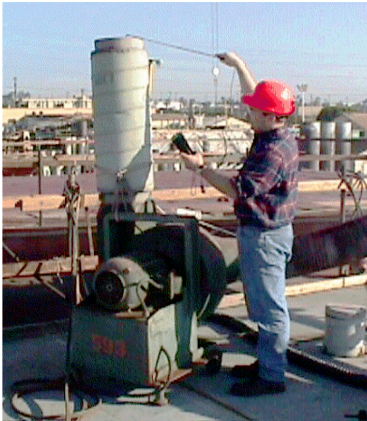
Photograph 2. Industrial Hygienist collecting ventilation measurements from a large, portable fume extraction unit
