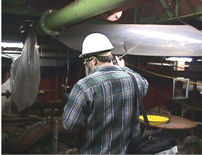
Photograph 1. Industrial Hygienist collecting ventilation measurements from ventilator supply air hose in a ship engine room
