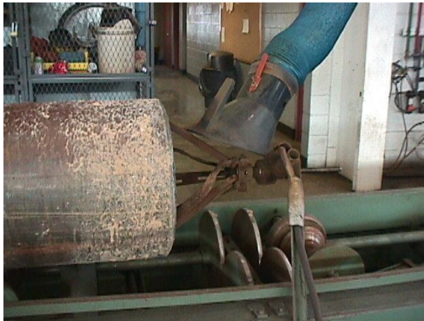
Photograph 5. Fixed fume extraction hose positioned directly above work to be performed
