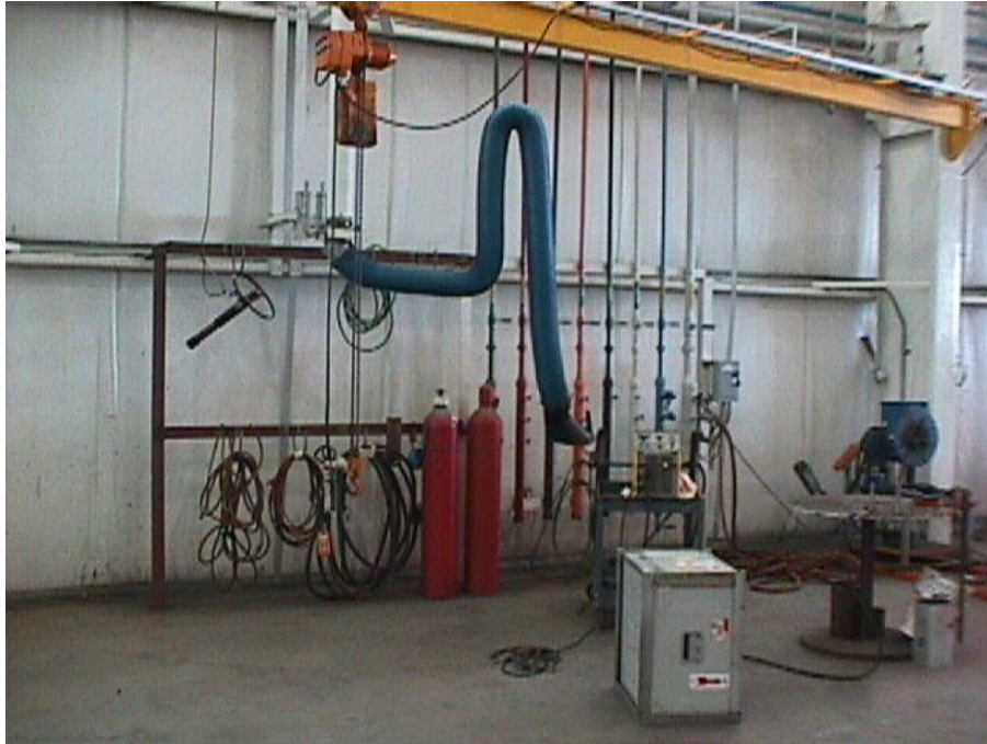
Photograph 6. Welding station equipped with portable fume extraction hose on articulating arm
