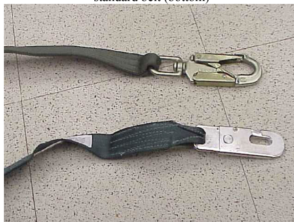
Fig. 3: Detail of standard CSB hook (bottom) and MARS CSB hook (top)
