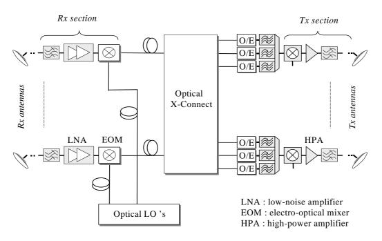
Fig. 6 : Schematic of an opto-microwave cross-connect repeater system
