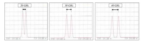
Fig. 2 : Optical spectra (in linear scale) of photonic LO's from 20 to 40 GHz
