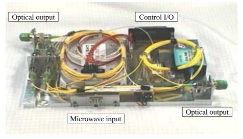
*Fig. 1 : Breadboard of the photonic local oscillator block*
