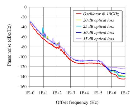
Fig. 3 : Experimental phase noise performance of a 20 GHz photonic LO distribution system versus optical losses
